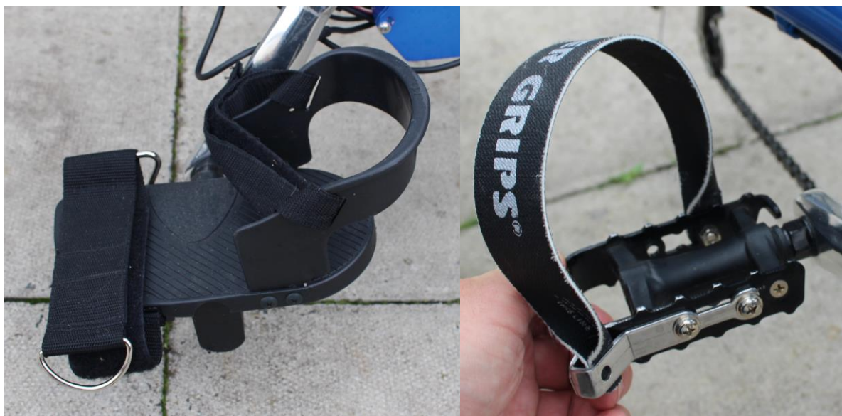
Figure 8: The self-levelling foot sandal with ankle support and pedal with a strap attached.
