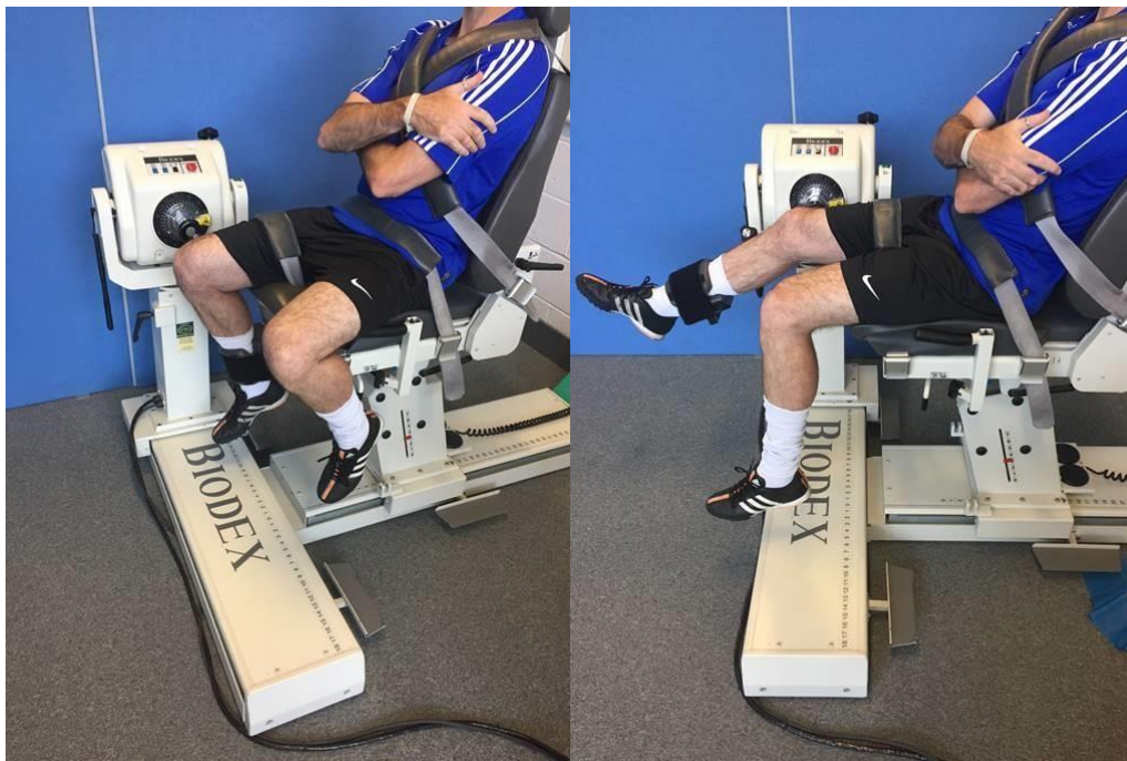
Figure 1.3 Image of the setup of the IKD for the testing protocol.
