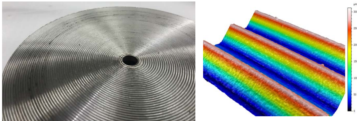
(a) (b) Figure 3: (a) Images of disk representing pressure plate (b) Measured surface at x5 magnification showing an area of approximately 6\text{ mm}^2
