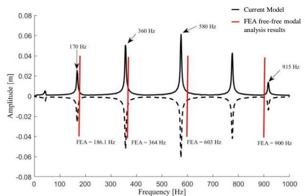
Figure 2: Frequency amplitude sweep for the bending modes in the x-z plane
