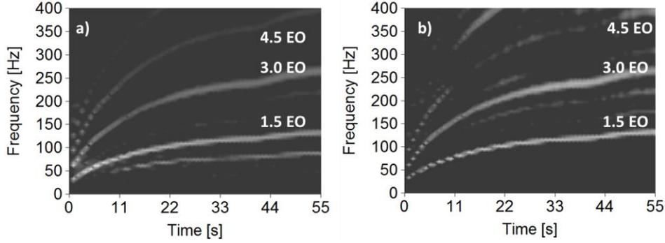
Figure 3: Continuous wavelet transform for: a) numerical and b) experimental transmission input shaft acceleration
