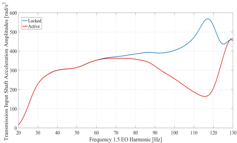
Figure 5: 1.5 EO acceleration amplitudes of transmission input shaft with locked and active NES ( $J_N = 8\%$  transmission input shaft inertia,  $k_N = 5 \times 10^5 \text{ Nm/rad}^3$ ,  $c_N = 0.001 \text{ Nms/rad}$ )
