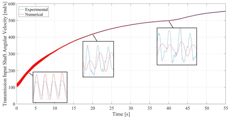
Figure 2: Comparison of the transmission input shaft velocity for numerical and experimental time histories
