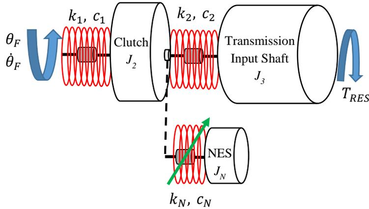
Figure 4: Schematic of the reduced powertrain model with a cubic nonlinear absorber
