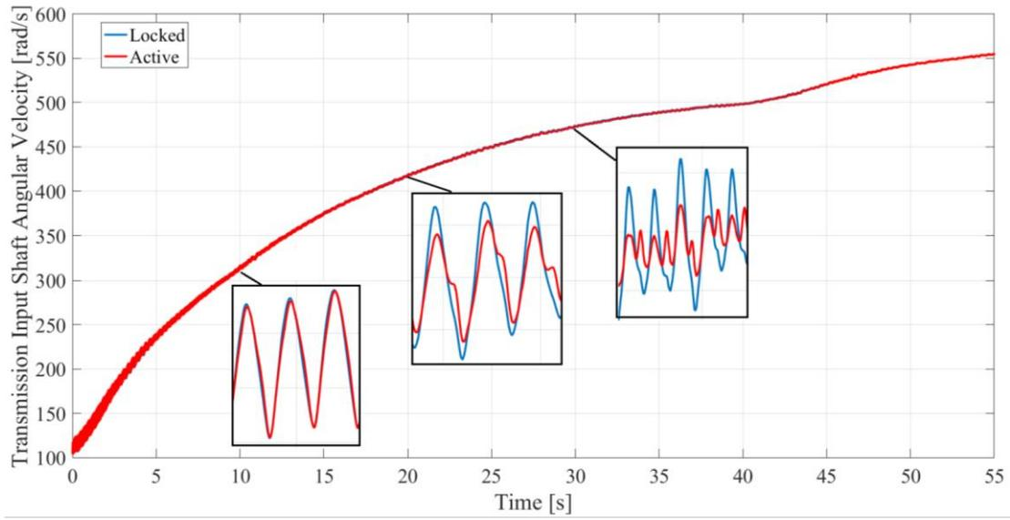
Figure 6: Comparison of transmission input shaft velocity for the systems with locked and active NES
