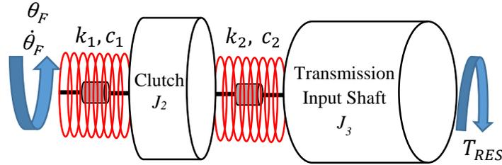
Figure 1: Schematic of the reduced powertrain model
