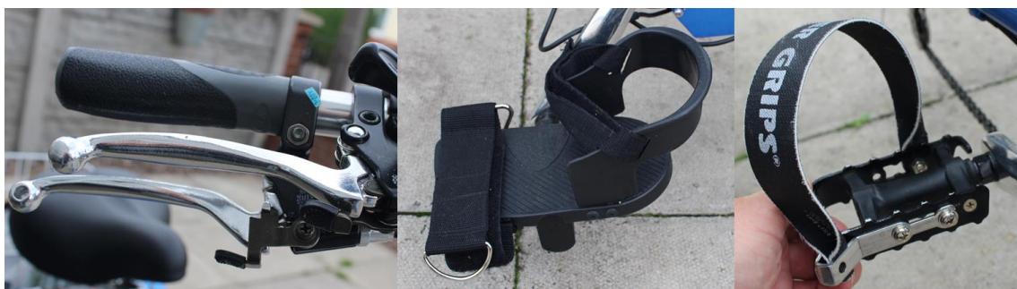
174 175 176 177 178 179 Figure 2: The adaptations available to the stroke survivors. From left to right - 180 repositioned breaks that could be operated simultaneously by the least effected side, 181 a self-levelling pedal with ankle support, and a pedal with a strap attached
