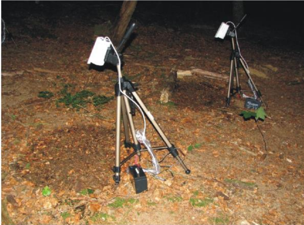
Fig. 1 Set-up for webcam recording of Lumbricus badensis behaviour at the soil surface in a beech/spruce-dominated forest at Belchen in the Schwarzwald area, Germany.
