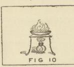
place some of the distillate (that is the liquid in the receiver) into a tin dish; stand it upon a tripod and gently warm it by means of a spirit the liquid lamp. as begins to warm, if alcohol is anv contained therein
