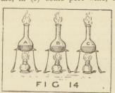
whiskey; on gently heating the flasks the alcohol contained in these liquids will be driven off, and will burn with flames of various size according to the quantity of alcohol present. Malt
