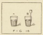
16; half fill the glasses with water. Pour on to glass (a) a little sweet oil. The oil will float on top of the water because it is lighter; that is to say that a glass of oil would not weigh so
