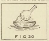
some burning alcohol, as shown in Fig. 20, the outside of the flask will become covered with moisture, so as to make the hand wet if passed over it. We may learn from these two experiments
