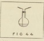
the flask, the other long enough to just pass through the In the flask put a little clear lime water. Place the short glass tube in the mouth and draw air through. Air will enter the long tube and
