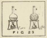
oil is placed. Both are ignited. Flask (a) will remain clean; flask (b) will be covered with soot. Another good quality of the alcohol is, that whilst it burns so freely it is not explosive like many inflammable substances.
