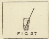
in Fig. 27, and gently breathe for a few minutes through the tube, allowing the breath to bubble through the water. We shall observe that the water, which was clear at starting, becomes turbid
