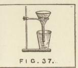
impurities by a filter, but it cannot be purified in that way from anything that is in solution. Mix some sugar and some sand with water; after well stirring pour it on to the filter, as shown in Fig. 37. This is an
