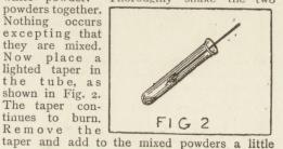
water. Now we can see at once that change takes place, for the powders begin to fizz and to effervesce, and on putting the lighted taper into the mouth of the tube it is at once extinguished.
