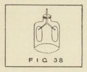
india-rubber bag is securely tied. The open bottom of the jar is now covered with a piece of leather. If the leather bottom is pushed up, air is squeezed out of the two bags and passes out of the glass tube. If the leather bottom is pulled down to the dotted line, air passes down the glass tube and inflates the two bags. This fairly represents the way in which we breathe. The
