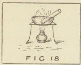
On making the water hot the alcohol will begin to boil before the water does, and it will pass completely away as vapour, nothing being left in the tube. Alcohol boils at 172°, but water boils at
