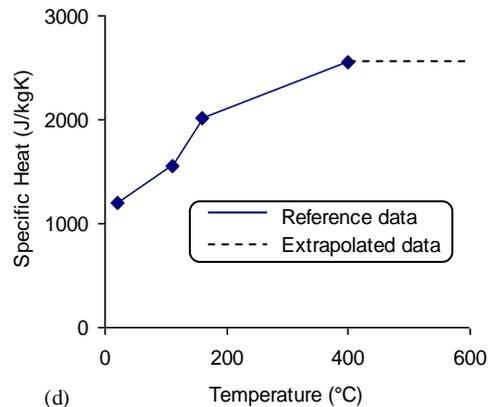
Figure 5. Thermal material properties of PS. a) EPS conductivity b) EPS specific heat c) XPS conductivity d) XPS specific heat.
