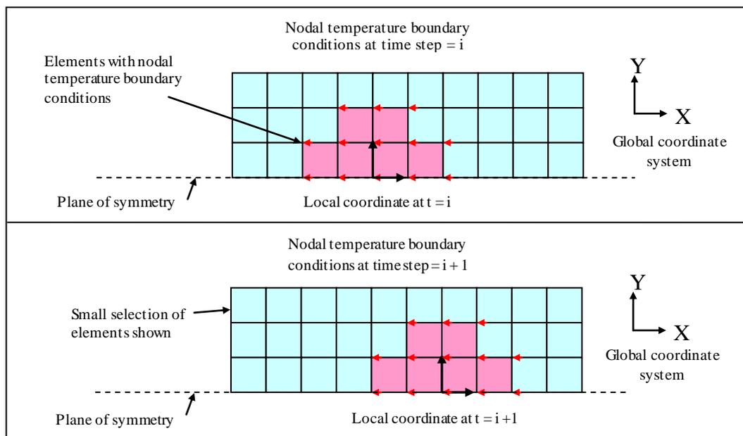
Figure 6. Nodal boundary conditions applied at nodes relative to the local coordinates for two successive time steps.
