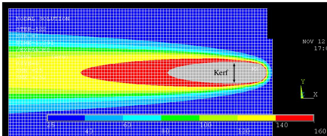
Figure 7. FEA temperature distribution for a hot-wire cut (EPS, 0.64 mm wire, 0.030 m/s).
