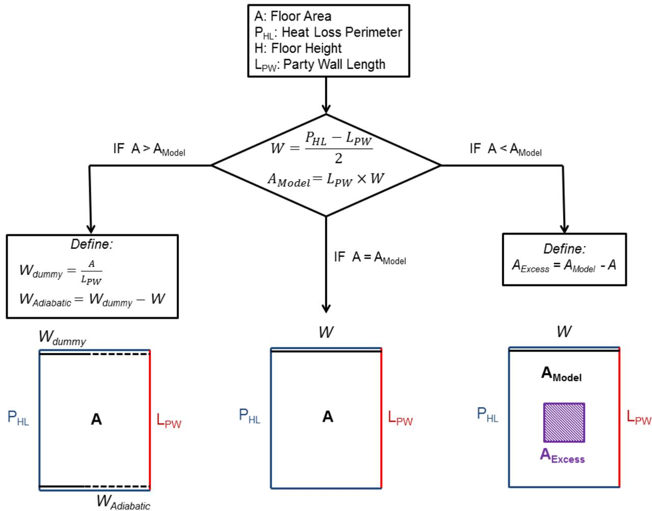
Figure 4.11 The methodology developed to model dwellings' geometry using the reduced data available in the modelling dataset
