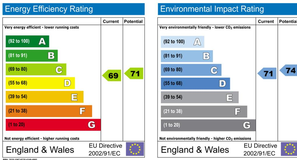
Figure 2.1 Example of EPC energy and EI ratings (RdSAP Manual, 2012)
