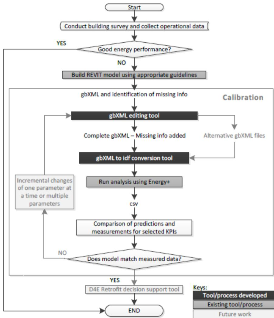
Figure 2.14 Structure and form of the BIM to BEM translator (Dimitriou et al., 2016)
