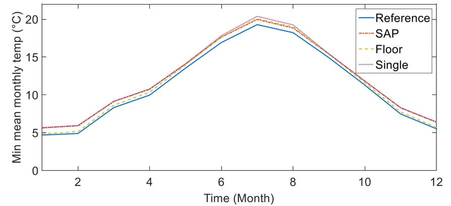
Figure 4.7 Internal temperatures of the three zoning strategies and the reference model under summer conditions. a) Maximum mean daily temperatures, b) minimum mean daily temperatures c) maximum mean monthly temperatures, d) minimum mean monthly temperatures
