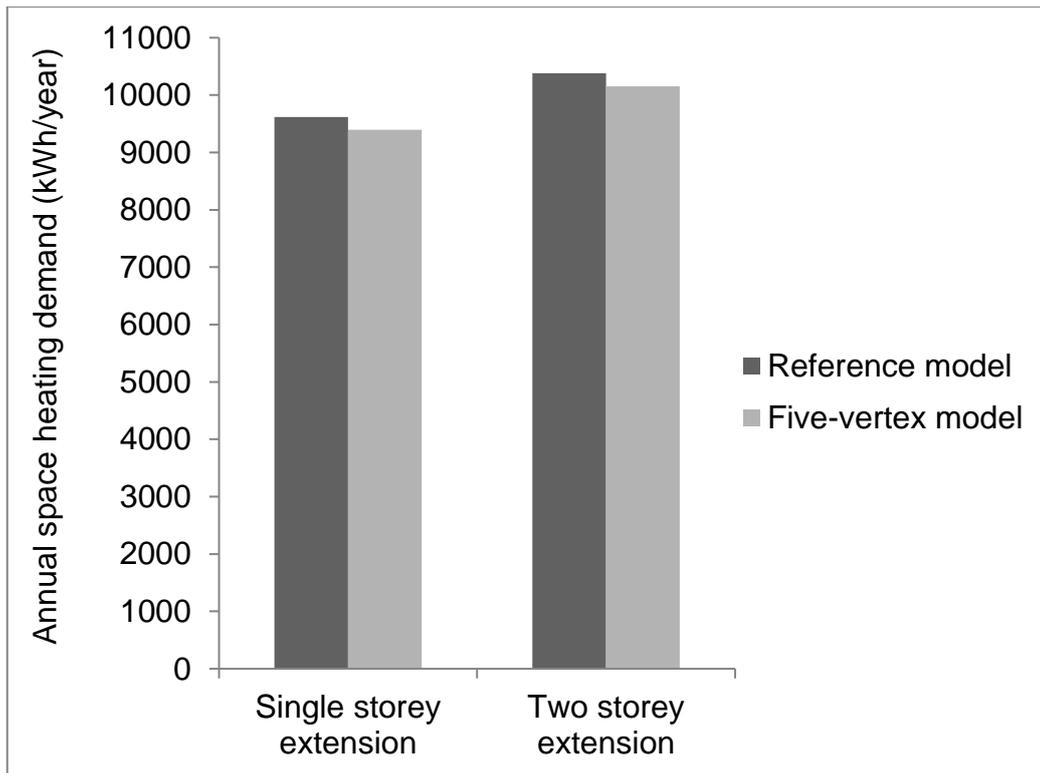
Figure 4.19 Annual space heating demand comparison of the reference model with extensions with five-vertex solution
