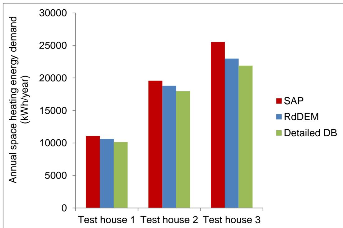
Figure 6.4 Comparison of the space heating demand from SAP, RdDEM and detailed DesignBuilder models of the three test houses
