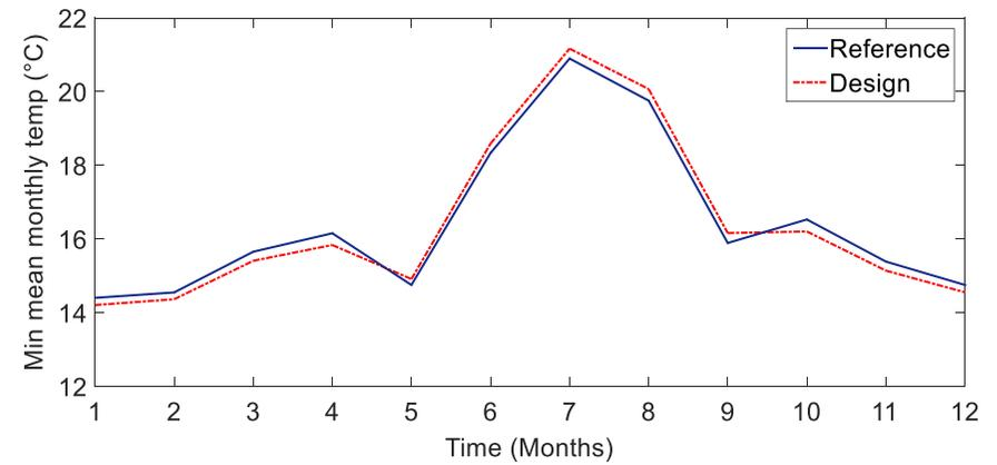
Figure 4.15 Internal temperatures of the reference geometry model and the design geometry model. a) Maximum mean daily temperatures, b) minimum mean daily temperatures c) maximum mean monthly temperatures, d) minimum mean monthly temperatures
