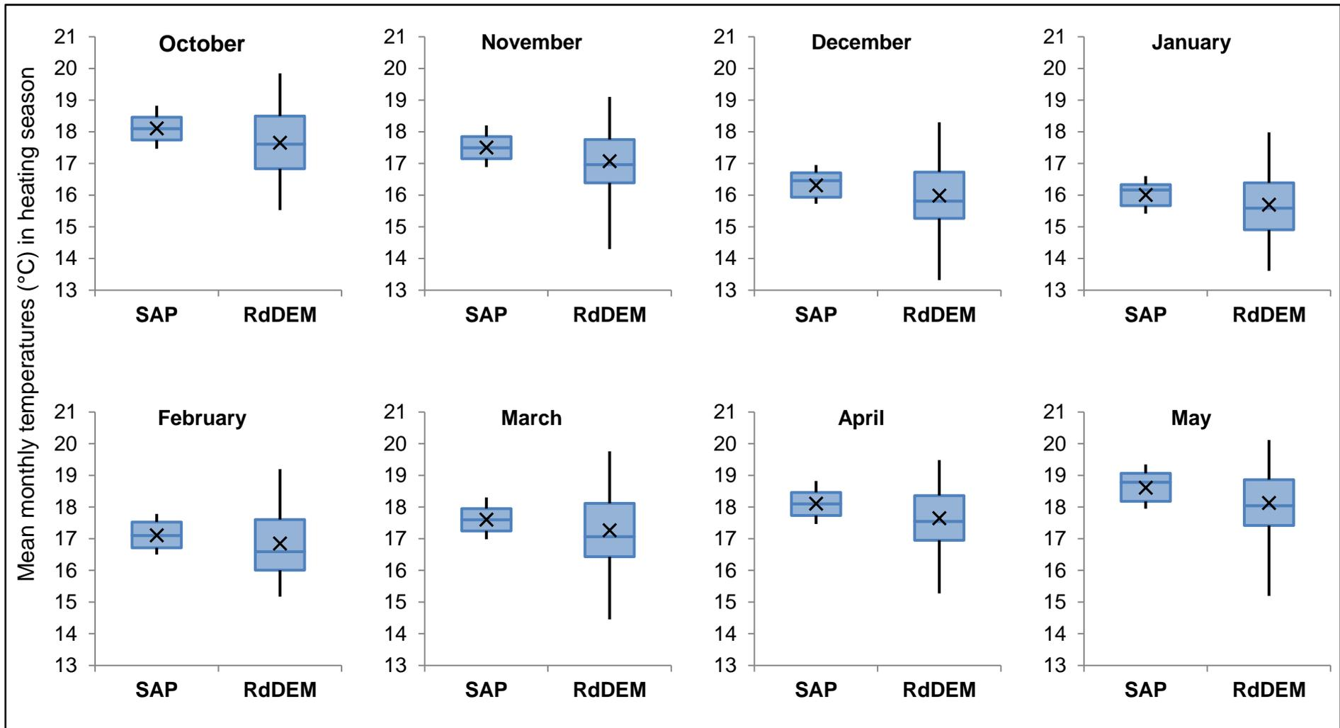
Figure 6.8 Comparison of the distributions of mean monthly internal air temperature
