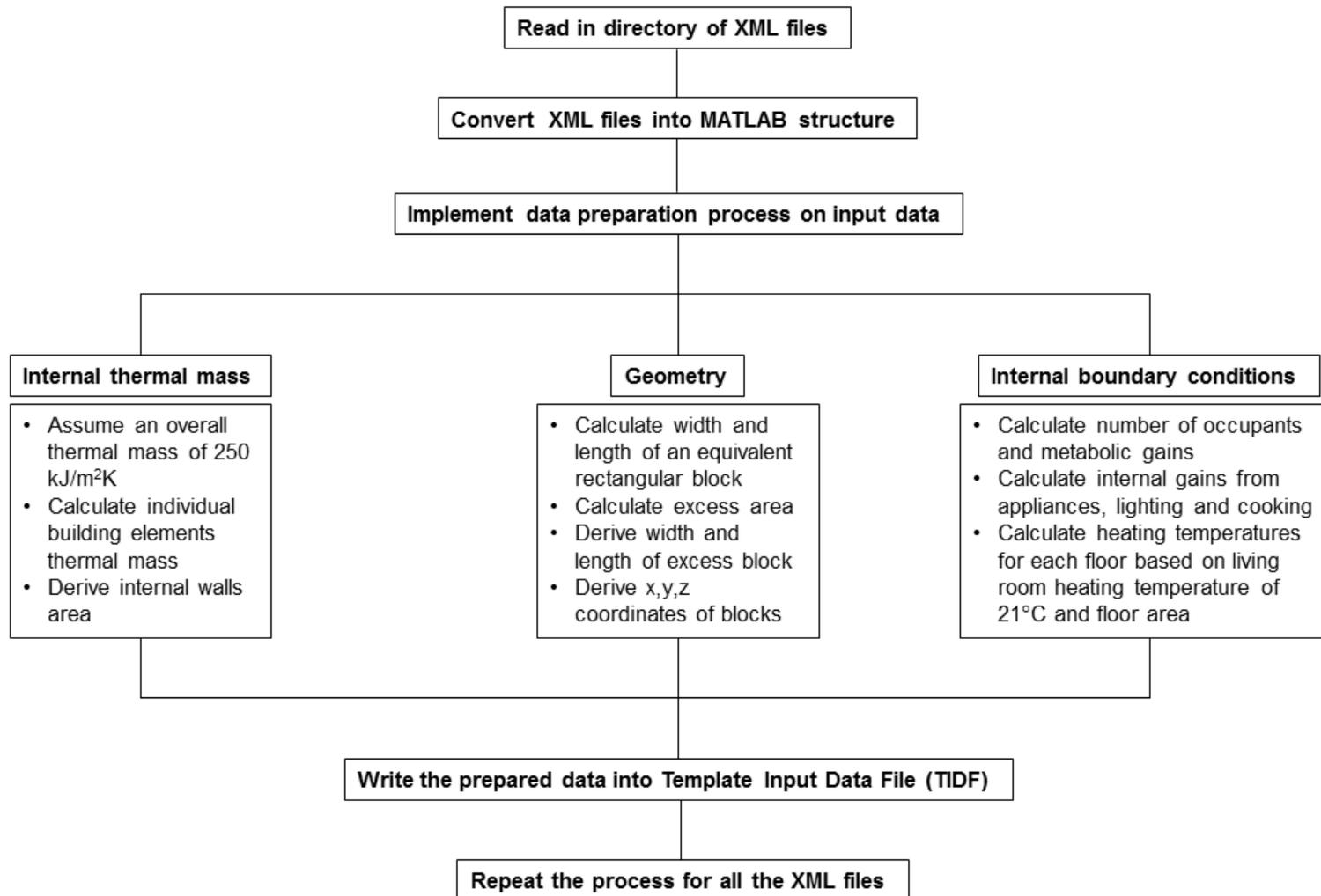
Figure 6.2 Translator framework to process varying data from XML files and write input data into Template IDF (TIDF)
