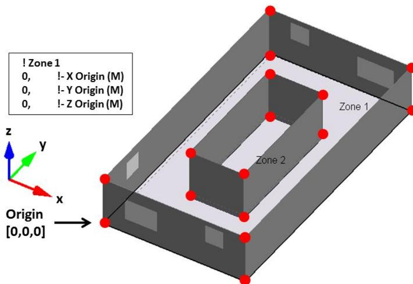
Figure 6.1 Geometrical layout of the dwellings' model with red dots showing the vertices of the rectangular blocks, the origin vertex and the IDF notation
