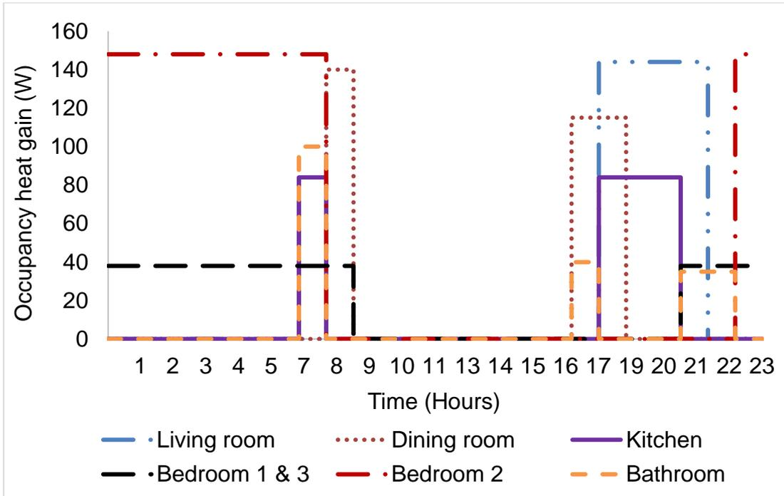
Figure 4.4 Occupancy gain profiles for individual rooms of A&P semi-detached house model
