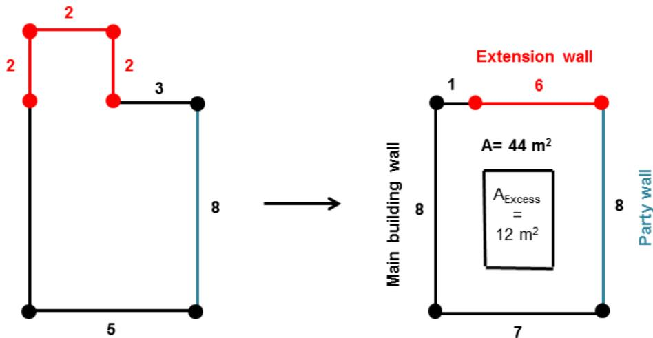
Figure 4.17 Modelling the extensions using five-vertex solution
