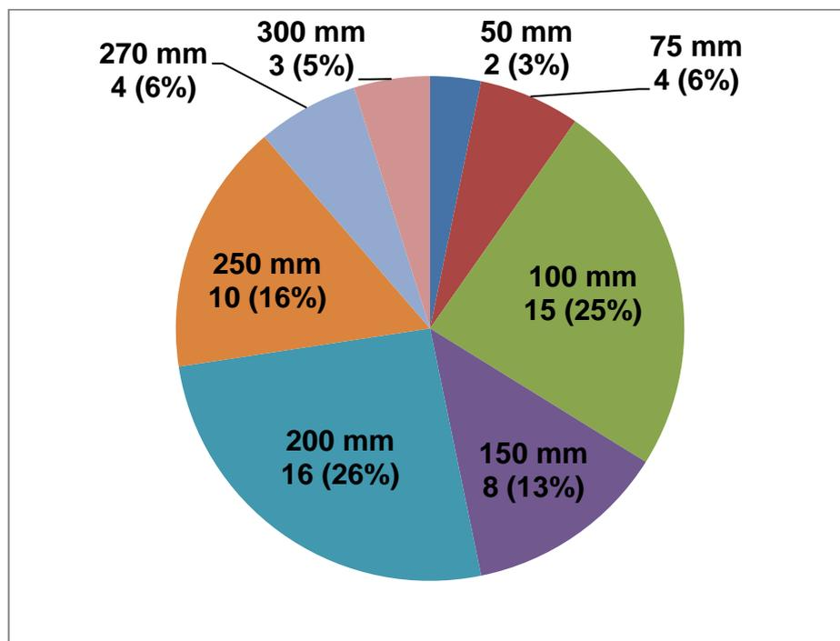
Figure 3.4 Dwellings distribution in the modelling dataset based on loft insulation thickness
