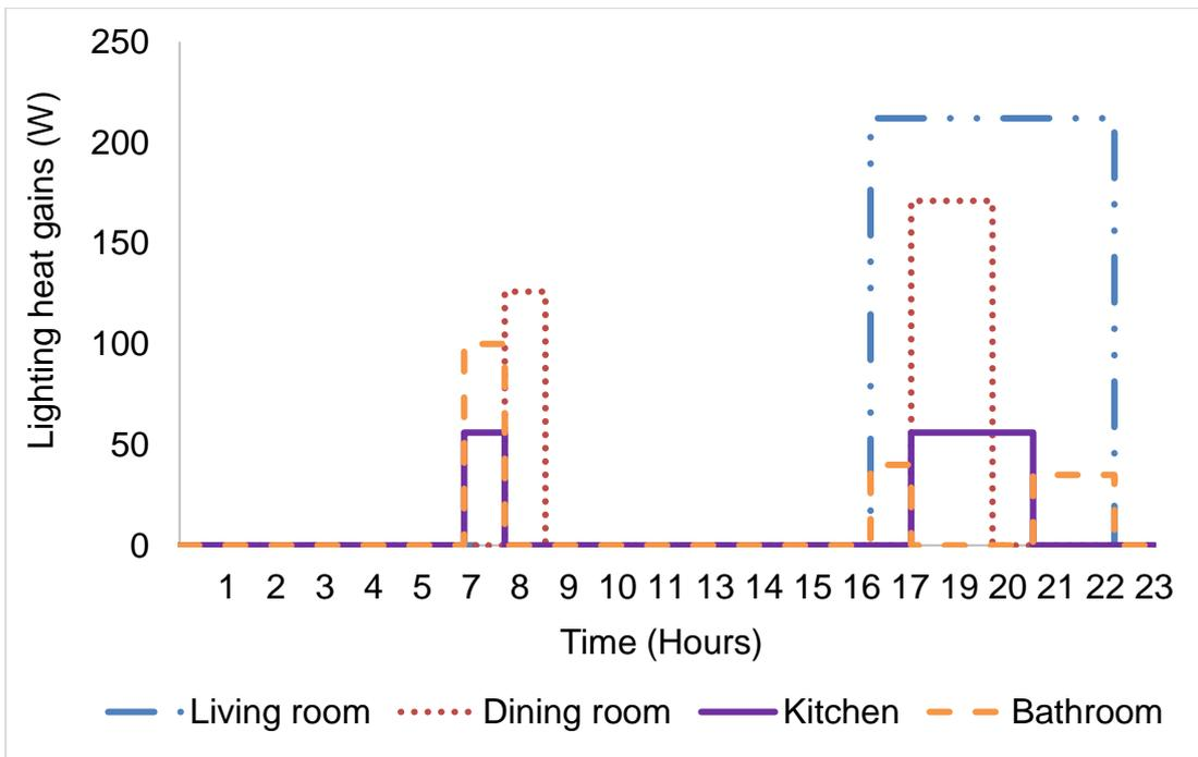
Figure 4.5 Lighting gain profiles for individual rooms of A&P semi-detached house model
