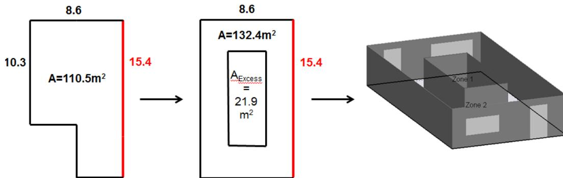
Figure 4.13 Transforming the reference geometry model to design geometry model
