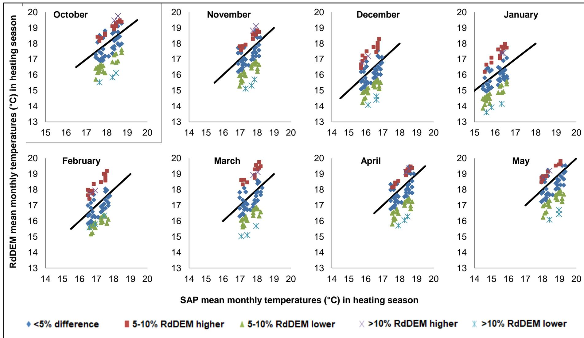
Figure 6.7 Comparison of RdDEM mean monthly internal temperature predictions to SAP (The black line represents  $x=y$ )
