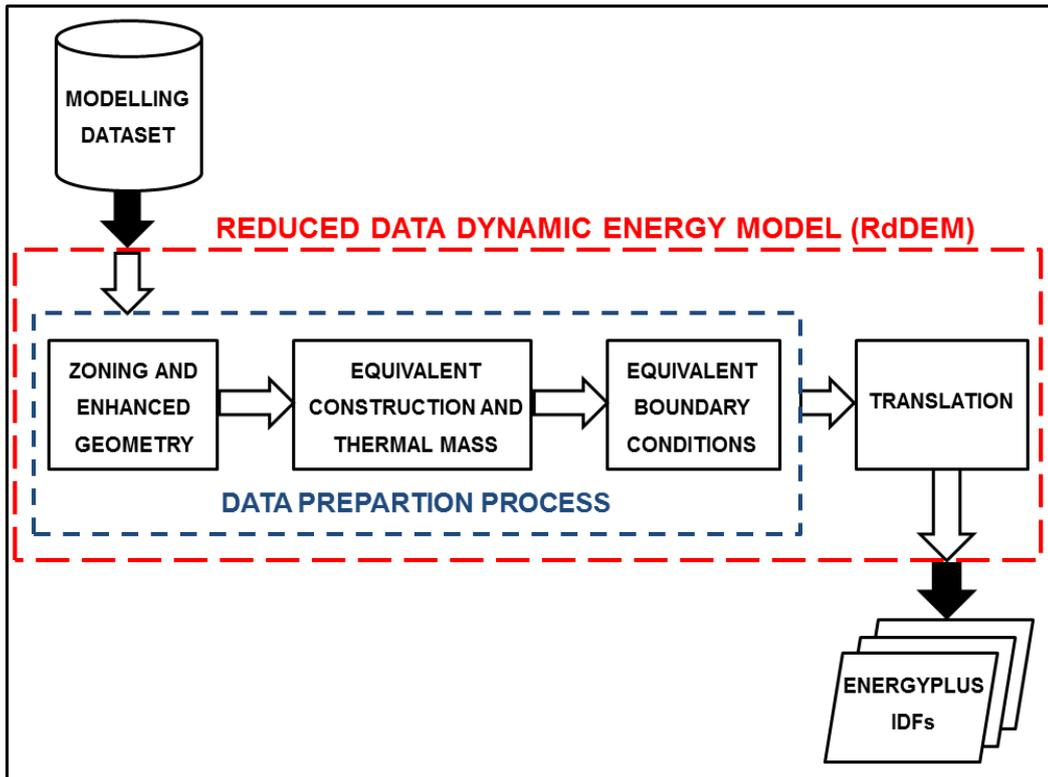
Figure 3.1 Overall structure and the modelling framework
