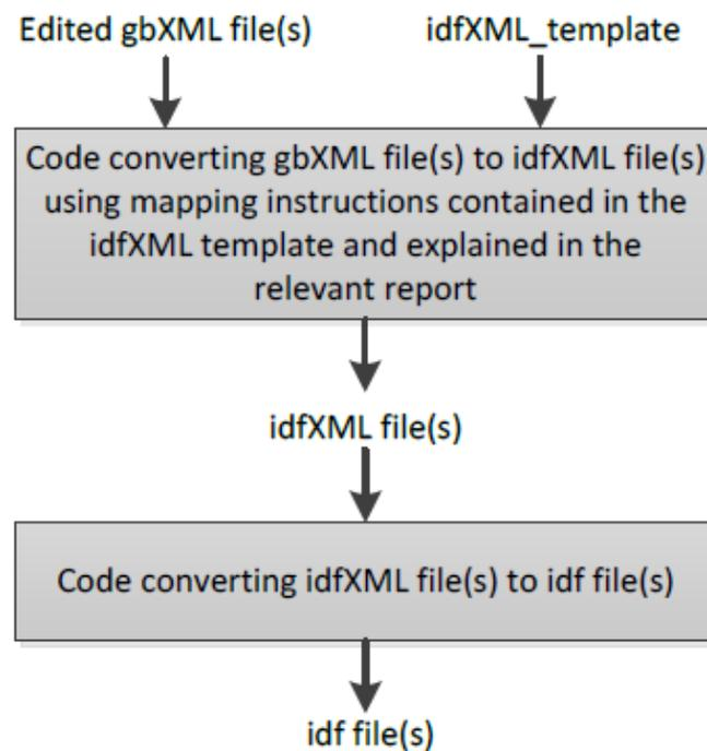
Figure 2.15 The translation process to convert gbXML files into EnergyPlus IDF files (Dimitriou et al., 2016)
