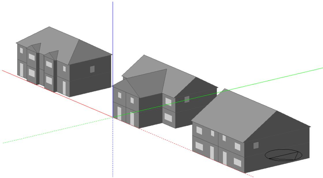
Figure 4.12 Left to right: The reference model, the reference geometry model and the design geometry model as created in DesignBuilder software package
