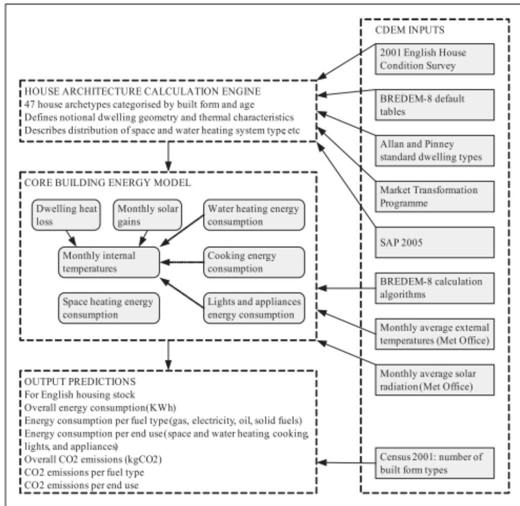
Figure 2.9 Structure and form of the CDEM (Firth et al., 2010)
