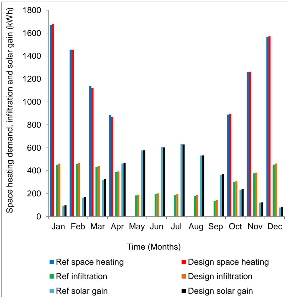
Figure 4.14 Monthly averaged space heating demand, external infiltration and solar gain estimates of the design geometry model compared to the reference geometry model
