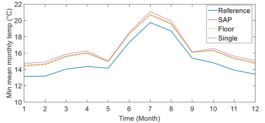
Figure 4.8 Internal temperatures of the three zoning strategies and the reference model under winter conditions. a) Maximum mean daily temperatures, b) minimum mean daily temperatures c) maximum mean monthly temperatures, d) minimum mean monthly temperatures
