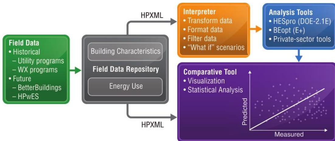
Figure 2.16 The translation process to convert HPXML files into various IDF formats (Polly et al., 2012)
