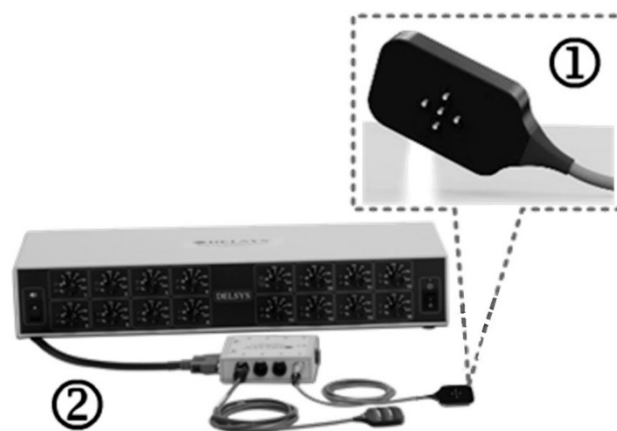
Figure 2. dEMG sensor (1); Delsys Bagnoli amplifier (2).
