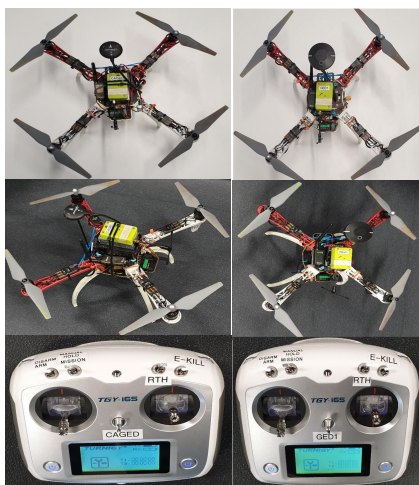
FIGURE 12: Hardware components of the rotary drones developed to test the system. CA Graffiti Equipped Drone (Left): Durandal (PX4) AutoPilot, DJI F450 Quadcopter Frame, DJI 960kv Motors x 4, DJI 4S 20A ESC x 4, TGY-IA6B 2.4GHz Receiver, TGY-I6S RC Controller, Pixhawk4 GPS Module, Raspberry Pi 4 (Companion Computer). Graffiti Equipped Drone (right): PixHawk2 Hex Cube (PX4) AutoPilot, DJI F450 Quadcopter Frame, DJI 960kv Motors x 4, DJI 4S 20A ESC x 4, TGY-IA6B 2.4GHz Receiver, TGY-I6S RC Controller, Here GPS Module and PilotAware Graffiti EC module.
