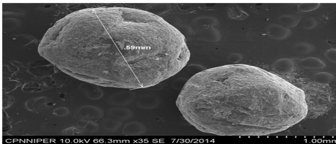
Fig. 7. Surface morphology of the optimized (F3) solid PB-SDEDDS.
