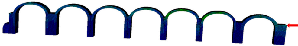
Fig. 21. Lateral point load acting on the right-hand side abutment of the structure.
