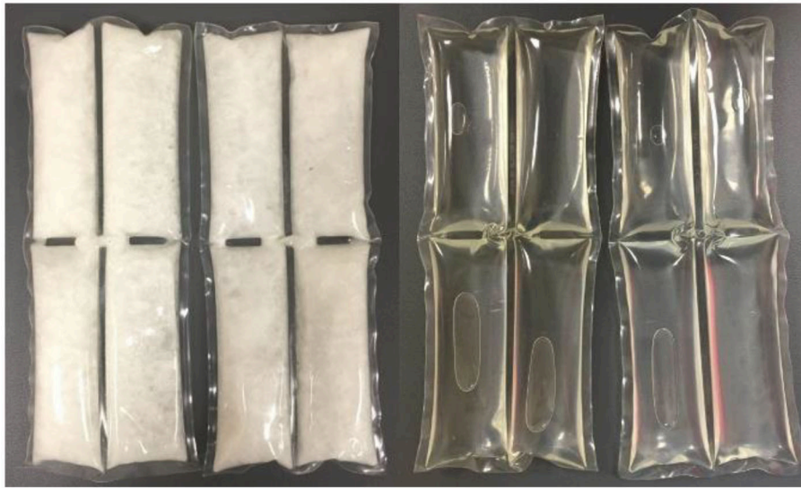
FIGURE 2 | Two Glacier Tek 15°C PCM packs in the frozen state (left), and in their melted state (right).
