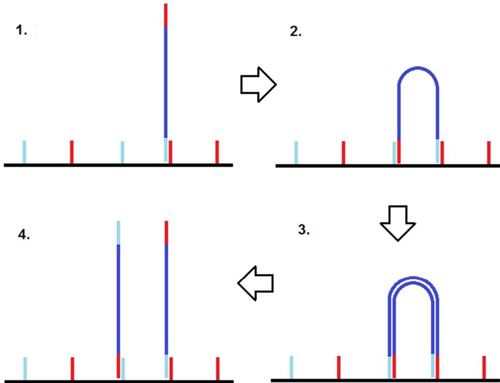
Figure 7: An illustration of the bridge PCR process used to generate clusters in sequencing by synthesis. 1. The library fragment is bound to the slide covered with oligonucleotides complementary to the library adapter sequences. 2. The library fragment forms a bridge shape. 3. PCR generates a complementary strand. 4. The result after multiple PCR cycles is a cluster of sequences attached to the slide which share the same sequence, some in the forward orientation, some reverse.
