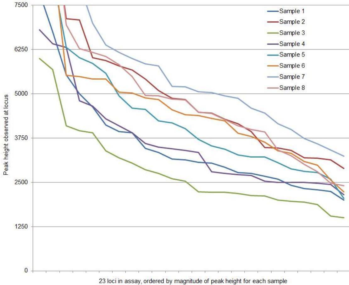
Figure 27: Chart of peak height observed at each locus in GlobalFiler CE-based inhibition analysis for each of the samples analysed. Sample numbers correspond to those shown in Table 14. Note that the horizontal axis displays each of the 23 loci in the multiplex, sorted by magnitude of coverage for each individual sample. The vertical axis measures the peak height seen at each locus for the sample.
