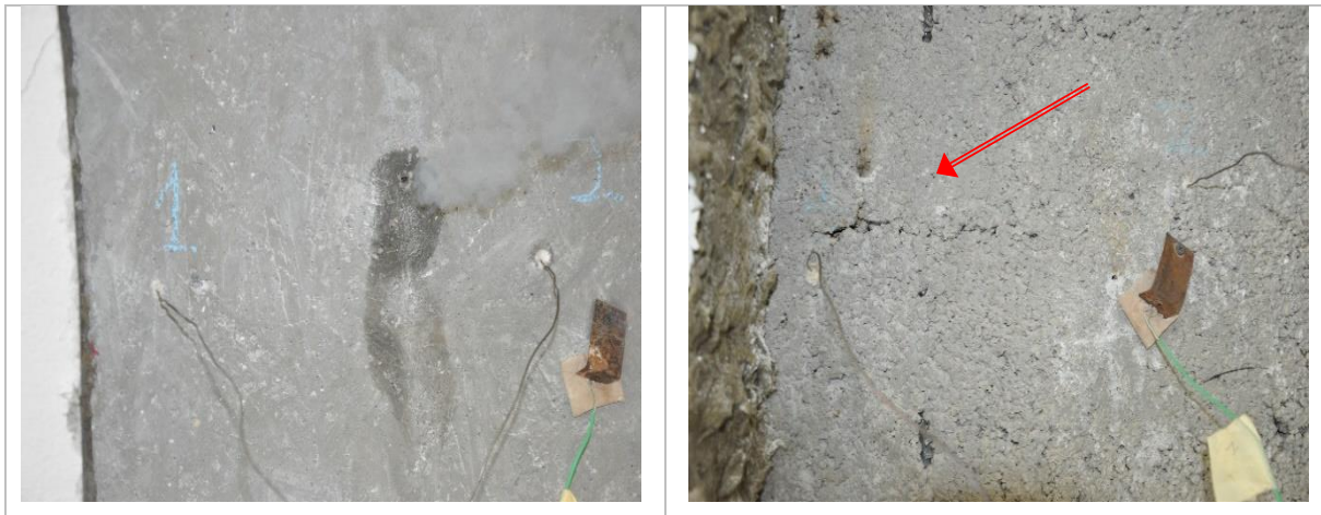
Figure 14. Dehydration (left, as manifested on the specimen placed on the right of the frame) and hairline cracking (right) during the test.
