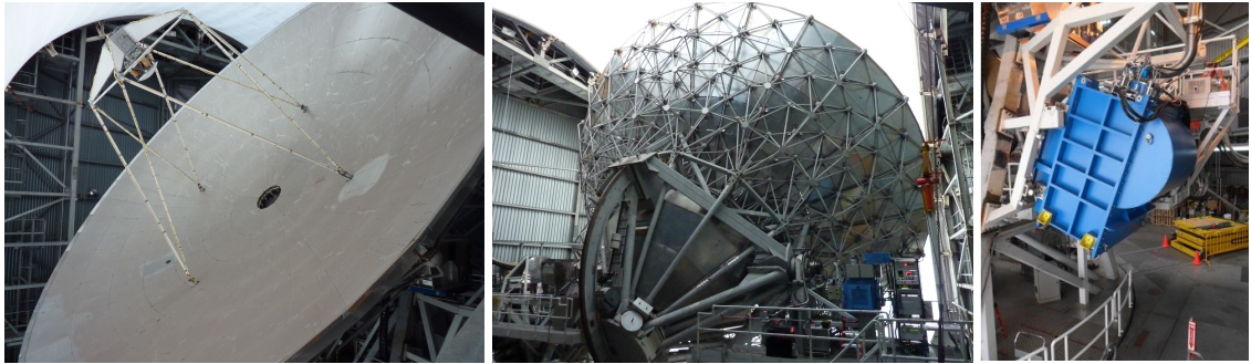
Figure 2.8: Components of JCMT and SCUBA-2. Left : Front of main dish and secondary reflector (credit: D.H.W. Glass). Centre : Rear of dish, showing linkages to stepper motors for dish panel alignment (credit: D.H.W. Glass). Right : SCUBA-2 detector housing (credit: EAO).
