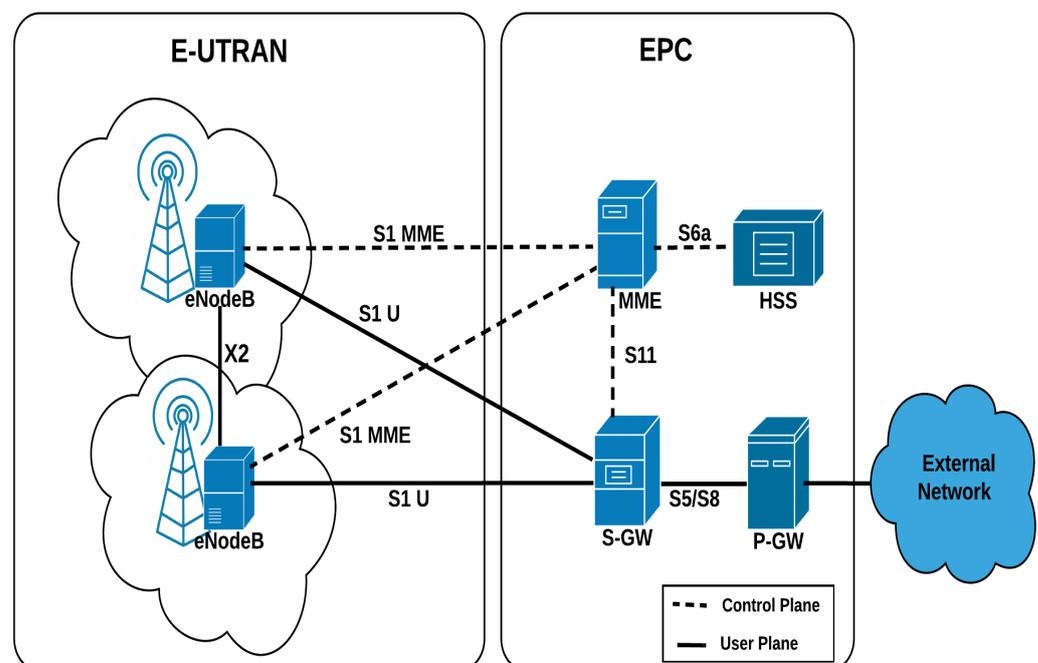
**Figure 1.** The Evolved Packet System (EPS) Network Elements.
