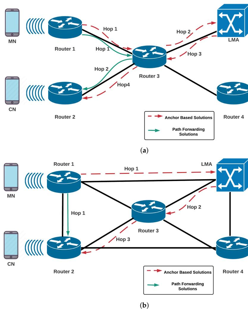
**Figure 5.** Packet Delivery Routes in Path Forwarding vs Anchor Based Networks. (a) Example Topology 1; (b) Example Topology 2.
