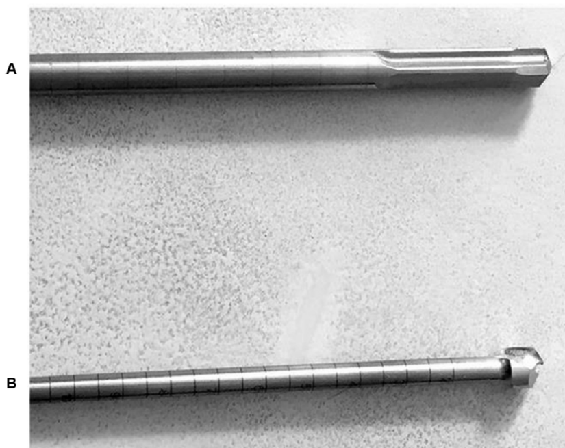
Fig. 2 (A) Fluted reamer featuring a wide reaming component that extends along its entire reaming length. (B) Acorn reamer with a narrower smooth shaft with wider reaming tip.
