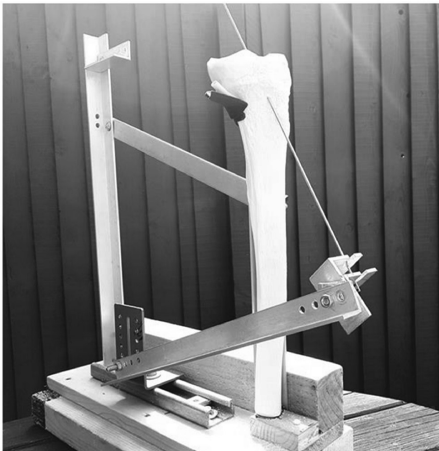
Fig. 1 Tibia Sawbones model on custom-made jig with guidewire in situ at the preset angle.
