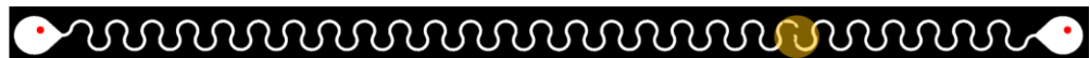
Figure 5. The output of the defect detection algorithm highlighting the disconnected resistance lines (yellow circle).
