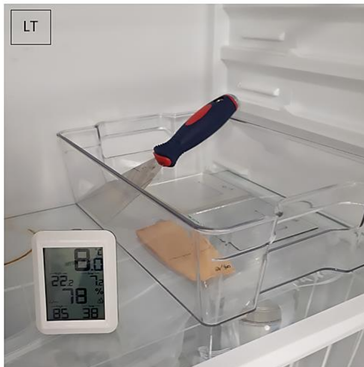
Figure 5.1: Selected surfaces stored at high temperature with moderate humidity (40 °C/50%) in the oven, and low temperature with high humidity (5 °C/78%) (LT) in the fridge. Temperature and humidity were monitored during the exposure period.
