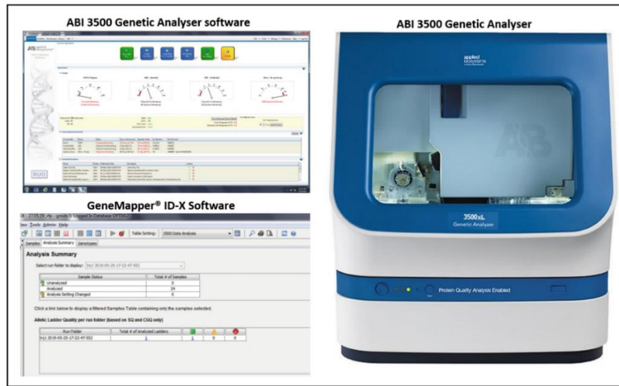
Figure 2.6: Capillary electrophoresis was performed on an ABI 3500 Genetic Analyser and the products were analysed using GeneMapper® ID-X Software.
