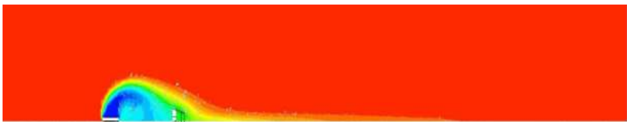
Figure 7.114: 2D view of temperature profile of heavy gas release source for a flat terrain with a solid fence as an obstacle at 1m/s velocity
