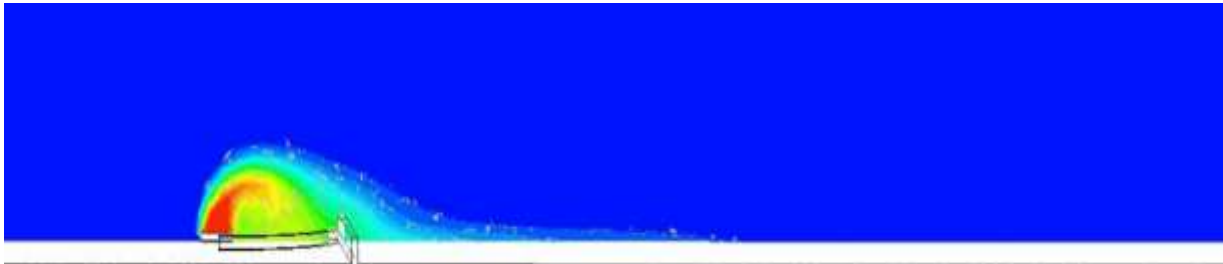
Figure 7.136: 2D view of flow rate profile of heavy gas release source for a flat terrain with a solid and a semi-circular fence as an obstacle with 1m/s velocity
