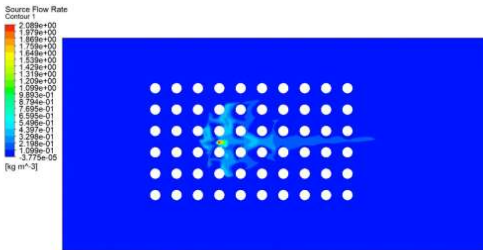
Figure 8.247: Concentration profile of the heavy gas dispersion with the release source located at the middle front of the group of gas storage tanks between the 3 rd and 4 th row from the bottom at 1m/s
