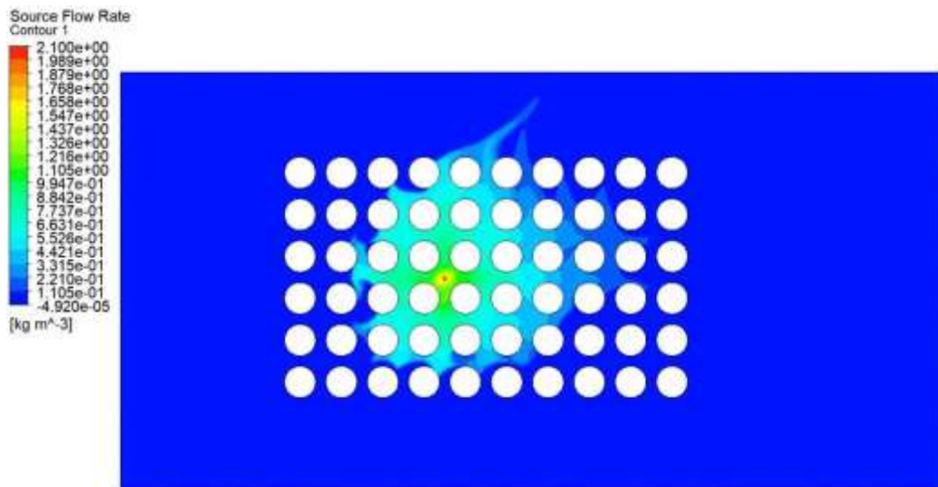
Figure 8.150: Concentration profile of the heavy gas dispersion with the release source located at the middle front of the group of buildings in the middle between the third and fourth rows at 1\text{m/s}
