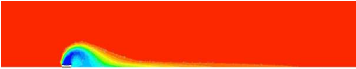
Figure 7.36: 2D view of temperature profile of heavy gas release source for a flat terrain with 1m/s velocity
