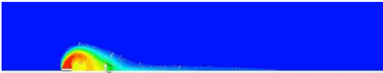
Figure 7.105: 2D view of concentration profile of heavy gas release source for a flat terrain with a solid fence as an obstacle with 1m/s velocity.
