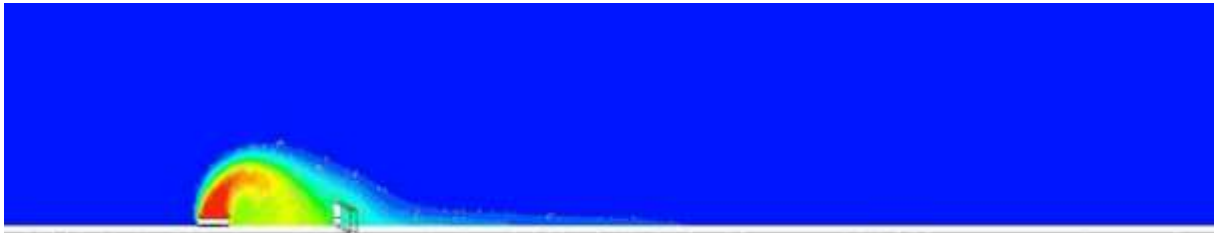
Figure 7.109: 2D-view of density profile of heavy gas release source for a flat terrain with a solid fence as an obstacle with 1m/s velocity
