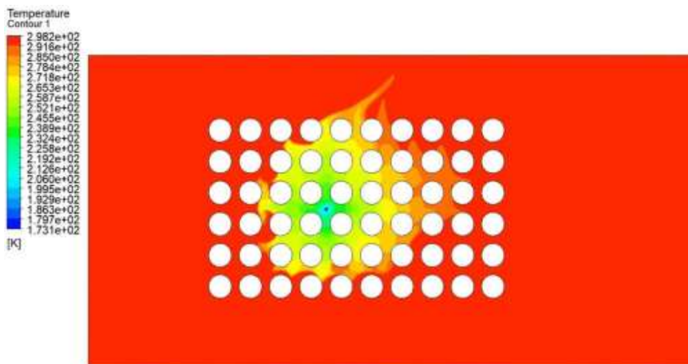
Figure 8.154: Temperature profile of the heavy gas dispersion with the release source located at the middle front of the group of buildings in the middle between the third and fourth rows at 1m/s.
