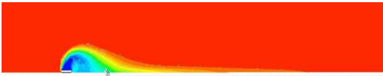
Figure 7.63: 2D view of temperature profile of heavy gas release source for a flat terrain with solid fence as an obstacle at 1m/s velocity
