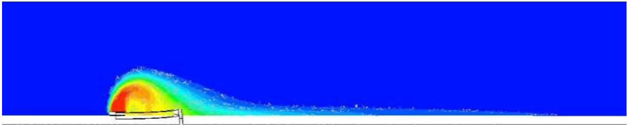
Figure 7.79: 2D view of concentration profile of heavy gas release source for a flat terrain with a solid and a semi-circular fence as an obstacle with 1m/s velocity
