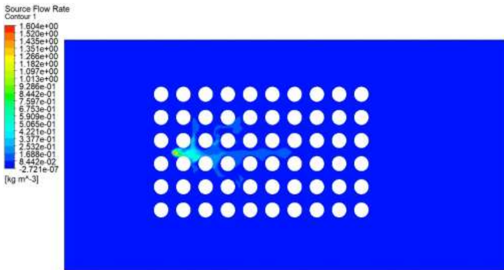
Figure 8.238: Concentration profile of the heavy gas dispersion with the release source located at the upwind front of the group of gas storage tanks between the first and second columns in the middle between the third and fourth rows at 1m/s .
