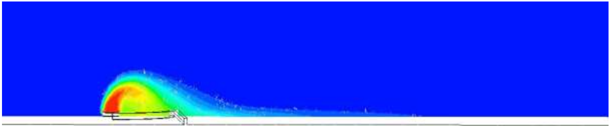
Figure 7.83: 2D view of density profile of heavy gas release source for a flat terrain with a solid and a semi-circular fence as an obstacle with 1m/s velocity
