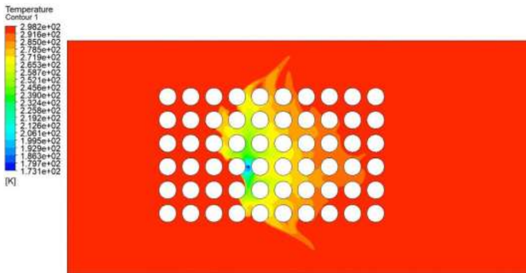
Figure 8.164: Temperature profile of the heavy gas dispersion with the release source located at the middle front of the group of buildings in the 3 rd row at 1m/s
