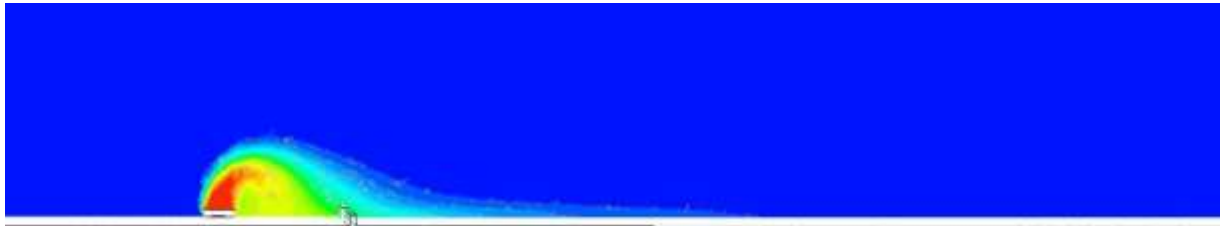
Figure 7.57: 2D-view of density profile of heavy gas release source for a flat terrain with a solid fence as an obstacle with 1m/s velocity
