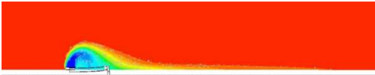
Figure 7.87: 2D view of temperature profile of heavy gas release source for a flat terrain with a solid and a semi-circular fence as an obstacle with 1m/s velocity
