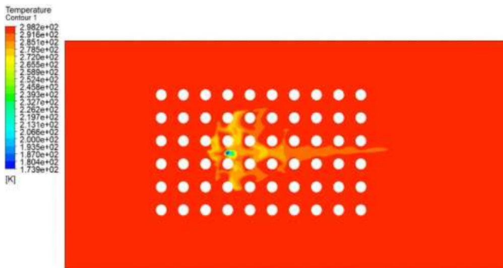
Figure 8.251: Temperature profile of the heavy gas dispersion with the release source located at the middle front of the group of gas storage tanks between the 3 rd and 4 th rows from the bottom at 1m/s
