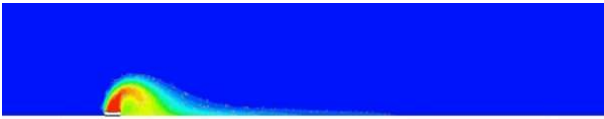
Figure 7.32: 2D-view of density of heavy gas release source for a flat terrain with 1m/s velocity
