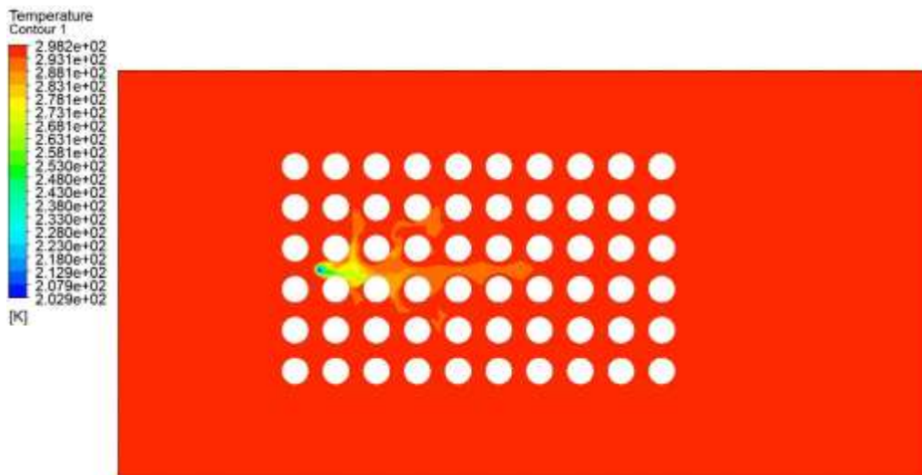
Figure 8.242: Temperature profile of the heavy gas dispersion with the release source located at the upwind front of the group of gas storage tanks between the first and second column in the middle between the third and fourth rows at 1m/s
