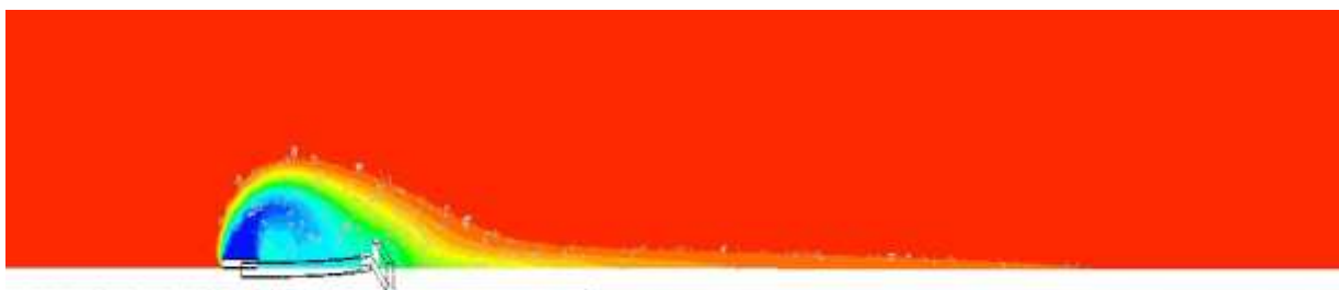
Figure 7.141: 2D view of temperature profile of heavy gas release source for a flat terrain with a solid and a semi-circular fence as an obstacle with 1m/s velocity
