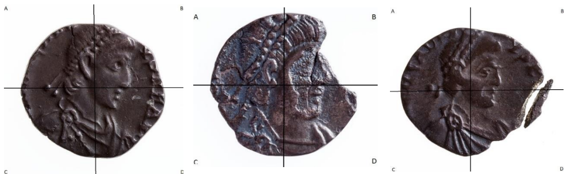
Figure 8.1.4-1. Images to show the different types of coin cracking. Coin ID 1386, possibly produced during production (left). Coin ID 1138, possibly during circulation or post-deposition (centre). Coin ID 1328, possibly during excavation or recovery (right).
