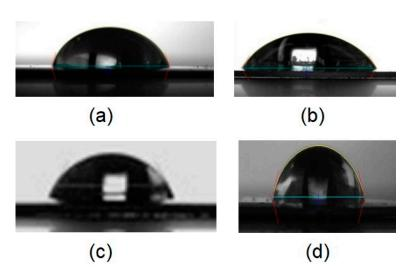
**Figure 1.** Contact angles of water on QCM-D discs coated with: (**a**) Nafion, (**b**) (Naf/Lys)<sub>6</sub>, (**c**) (Naf/CDot)<sub>6</sub>, and (**d**) (Naf/Lys/CDot/Lys)<sub>3</sub>. Subscript number refers to the number of bior trilayers. (**a**,**b**) adapted from [23].
