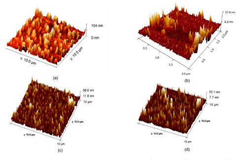
**Figure 2.** AFM of QCM-D crystals coated with: (**a**) Nafion, (**b**) (Naf/Lys)<sub>6</sub>, (**c**) (Naf/CDot)<sub>6</sub>, and (**d**) (Naf/Lys/CDot/Lys)<sub>3</sub>. Subscript number refers to the number of bi- or trilayers. (**a**,**b**) adapted from [23].
