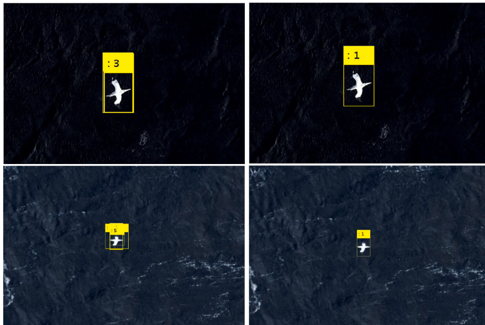
Fig. 13. Two magnified gannet objects detected by several detectors (left) and counted only once (right).
