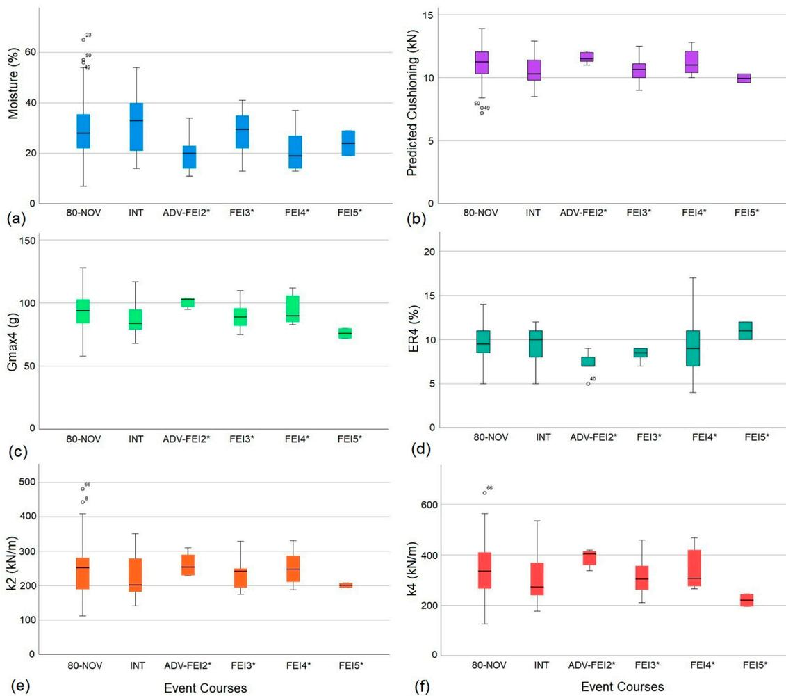
**Figure 2.** Boxplots of data from 2021 and 2022 eventing season (81 event courses) showing data for (a) moisture (%), (b) predicted cushioning (kN), (c) impact acceleration at 4 m/s (Gmax4) (g), (d) coefficient of restitution at 4 m/s (ER4) (%), (e) stiffness at 2 m/s (k2) (kN/m), and (f) stiffness at 4 m/s (k4) (kN/m) separated by course levels. Abbreviations: Novice (NOV), Intermediate (INT), Advanced (ADV), Fédération Equestre Internationale (FEI).
