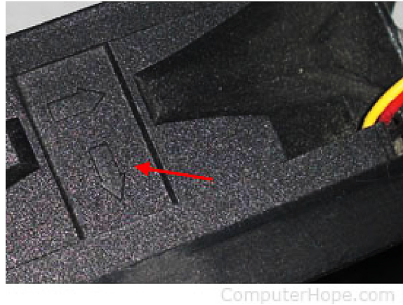
Fig. 6. Signs on ventilator specify fan blades rotation and airflow direction [7].
