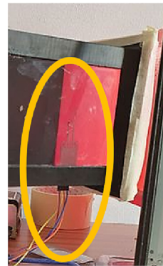
Fig. 7. Rev. P – hot wire anemometer with temperature sensor and its location in the wind tunnel [6,8].
