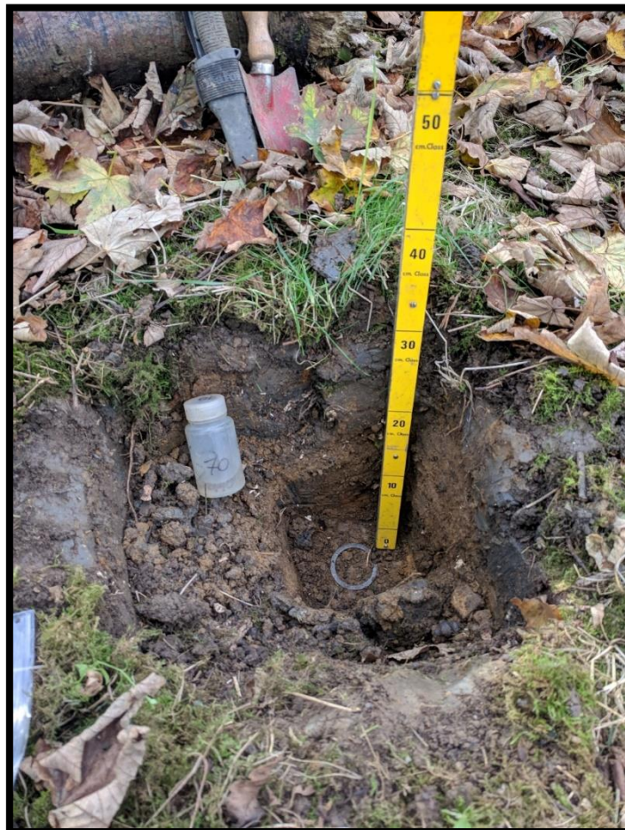
FIGURE 4.2 – Example of pit used for bulk density (BD) and earthworm sampling. A 30 x 30 x 30 cm volume of soil was excavated, and hand sorted for earthworms. Following this, a further 10 cm depth of soil material was excavated for BD sampling. The deepest BD core (30-50 cm) was extracted from the base of the pit.
