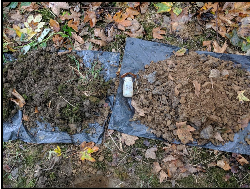
FIGURE 7.10 – Soil described as ‘sandy brown earth’ excavated from Winterton in October 2018. The left-hand soil is the upper 0 – 10 cm topsoil and is darker and blacker suggesting higher organic matter content. The right-hand soil is browner and lighter, matching descriptions by previous authors of ‘sandy brown earth’ (Drobig, 1999; Hislop and Harding, 1999).
