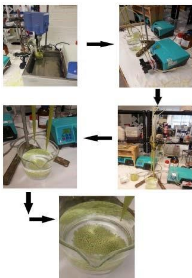
Figure 2.5 Synthesis of AMP/PAN beads by gravity dropping. Taken from P. Kavi. [10]
