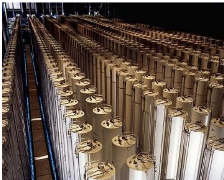
Figure 1.1.4 Centrifuges used in the enrichment process [10]
