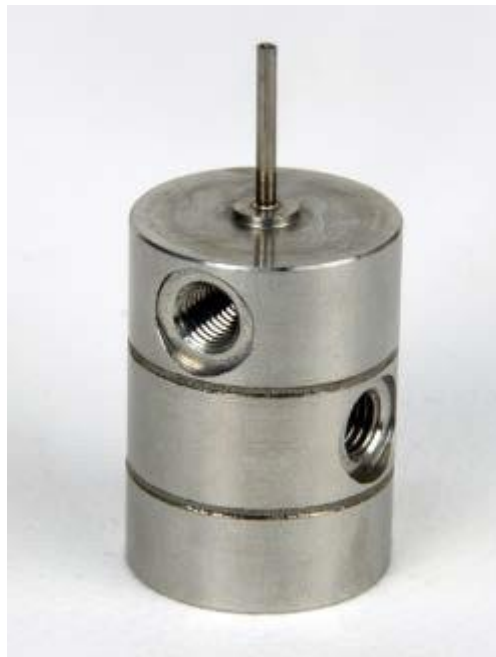
Figure 2.8 2-Layer sealed coaxial needle with threaded luer lock fastenings for gas and mixture feed inlets
