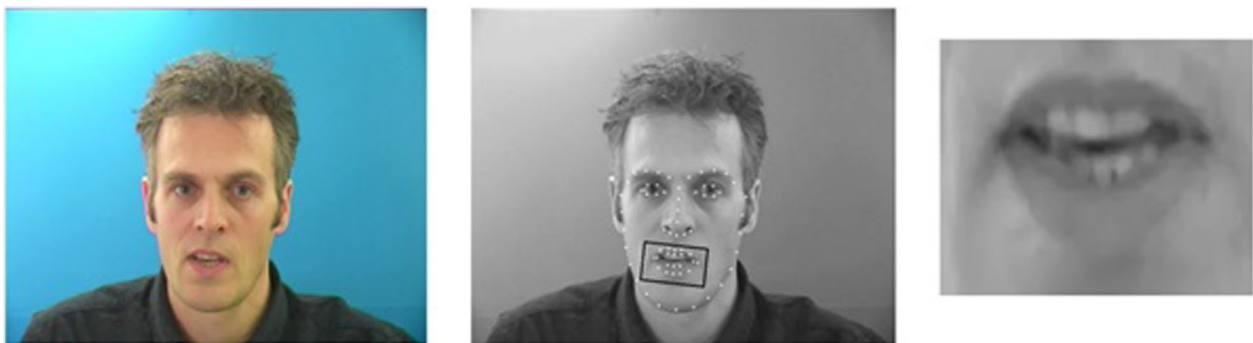
Fig. 1 Illustration of automatic detection and extraction of the lip region from an image
