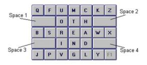
Figure 3: The OPTI keyboard layout
