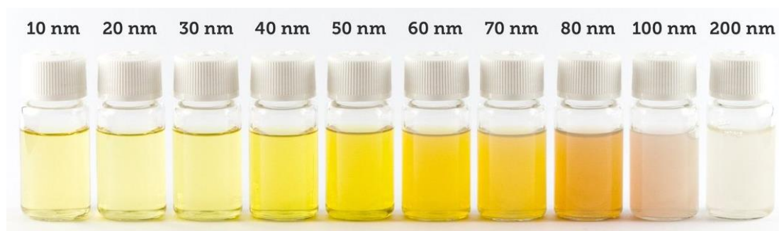
Figure 2.4: Dispersion of different sized citrate coated AgNPs (NanoComposix, 2019)
