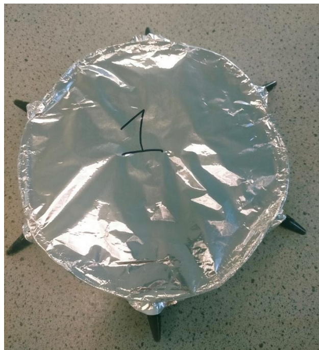
Figure 7.10: Example of food choice chamber (20 cm \phi ) with aluminium foil cover in place, (author's image)
