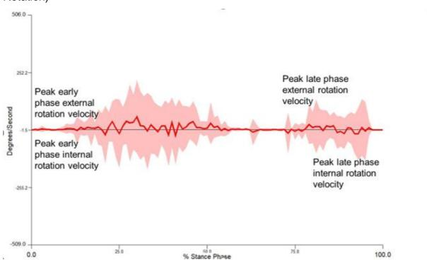
Figure 4.12 Tibial Angular Velocity in the Transverse Plane (Internal/External Rotation)
