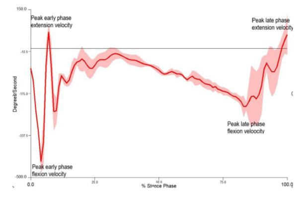
Figure 4.11 Tibial Angular Flexion/Extension Velocity in the Sagittal Plane
