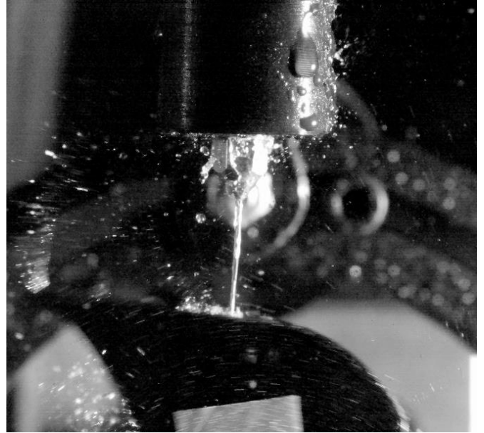
Figure 11 Secondary impact on the blade with a jet flow rate of 0.3 L/min
