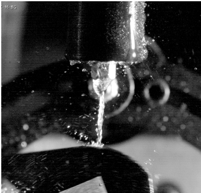
Figure 8 Corona Splashing on the upper blade surface with a flow rate of 0.22L\min
