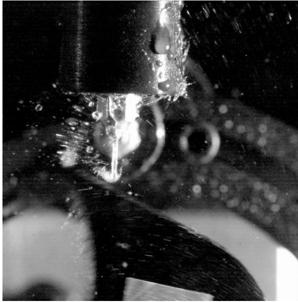
Figure 10 Jet disrupted after initial impact with a jet flow rate of 0.3 L/min
