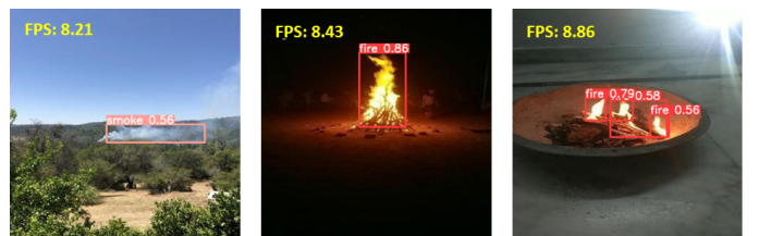
Fig. 6. Evaluation on the Raspberry Pi platform: the detection result of the image obtained in real time from the web camera, with the live detection frame rate in the top left corner of the detection screen.
