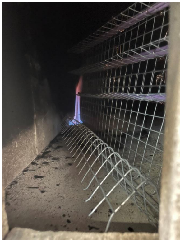
Figure 50: Picture of the reduced scale cable set up used in the flashover box
