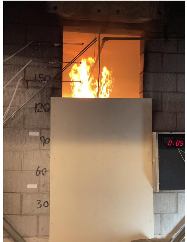
Figure 45: Diagram and picture of the door used to control the ventilation during under-ventilated tests.
