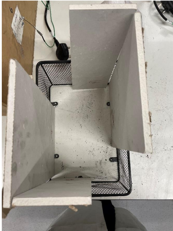
Figure 49: Picture of the reduced scale SBI rig set up in the flashover box.
