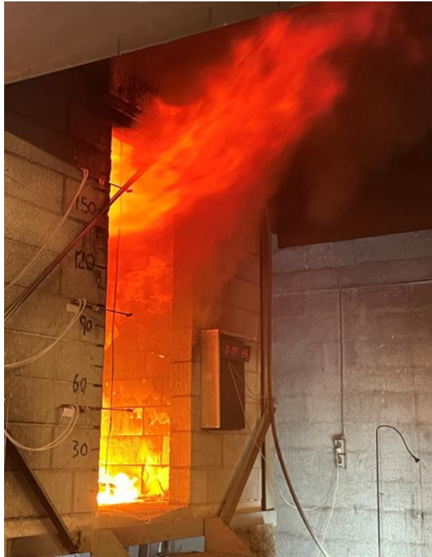
Figure 118: Picture taken approximately 300 seconds into the polyurethane (2x SBI) ISO 9705 room test.
