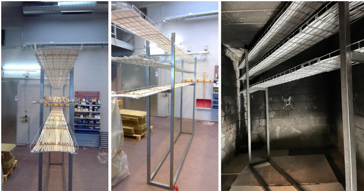
Figure 91: Picture of the cable trays set up on a stainless steel holder for testing in the ISO 9705 room corner. The ISO 9705 propane burner, while not visible, is below the end of the cable trays in the corner.
