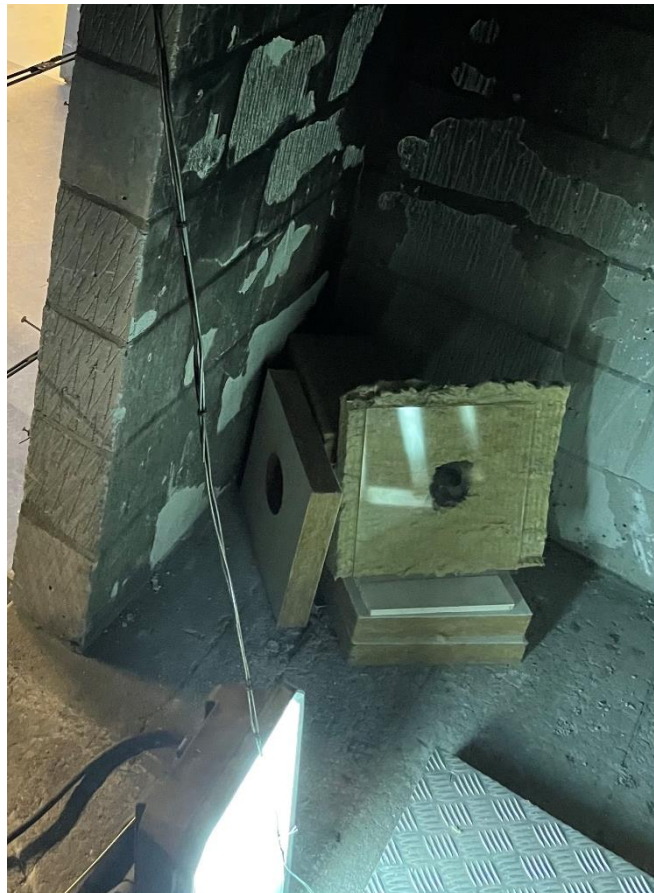
Figure 56: Picture of the camera set up to record the inside of the ISO room corner test protected by Rockwool and heat proof glass
