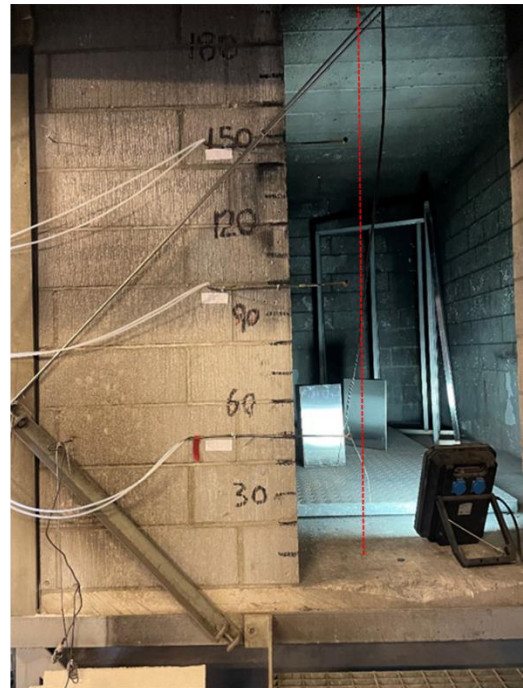
Figure 52: Diagram and picture of the placement of McCaffrey probes and thermocouple tree for air velocity and temperature measurements
