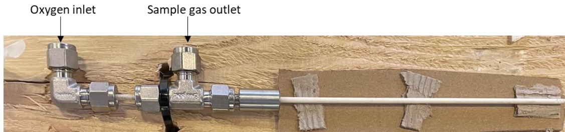
Figure 30: Labelled picture of the ceramic tube and air inlets and sample mixture outlets in the phi meter.
