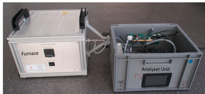
Fig. 6. Photograph of Phi meter furnace and analyser unit.
