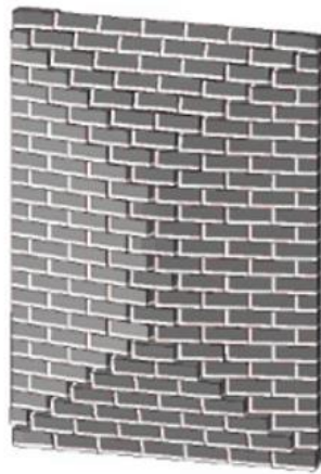
Figure 2. Out-of-plane failure pattern of a wall subjected to blast loading.
