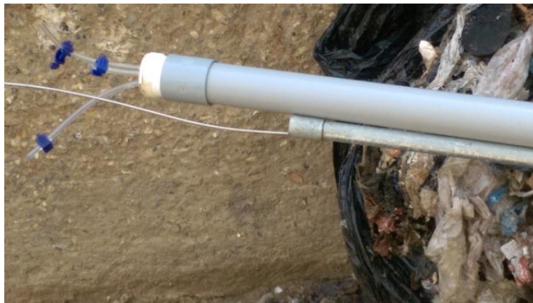
Figure 197: Gas sample tubes for test No18
