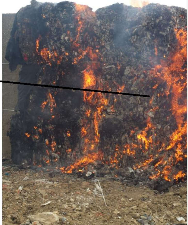
Figure 139: Test No 10 (table 2) RDF Stack degradation.
