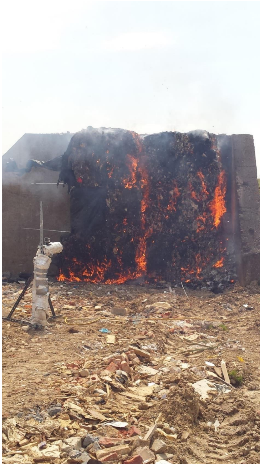
Figure 137: Test No 10 (table 2) area of intense flame is observed to generate in the gaps between the stacks.
