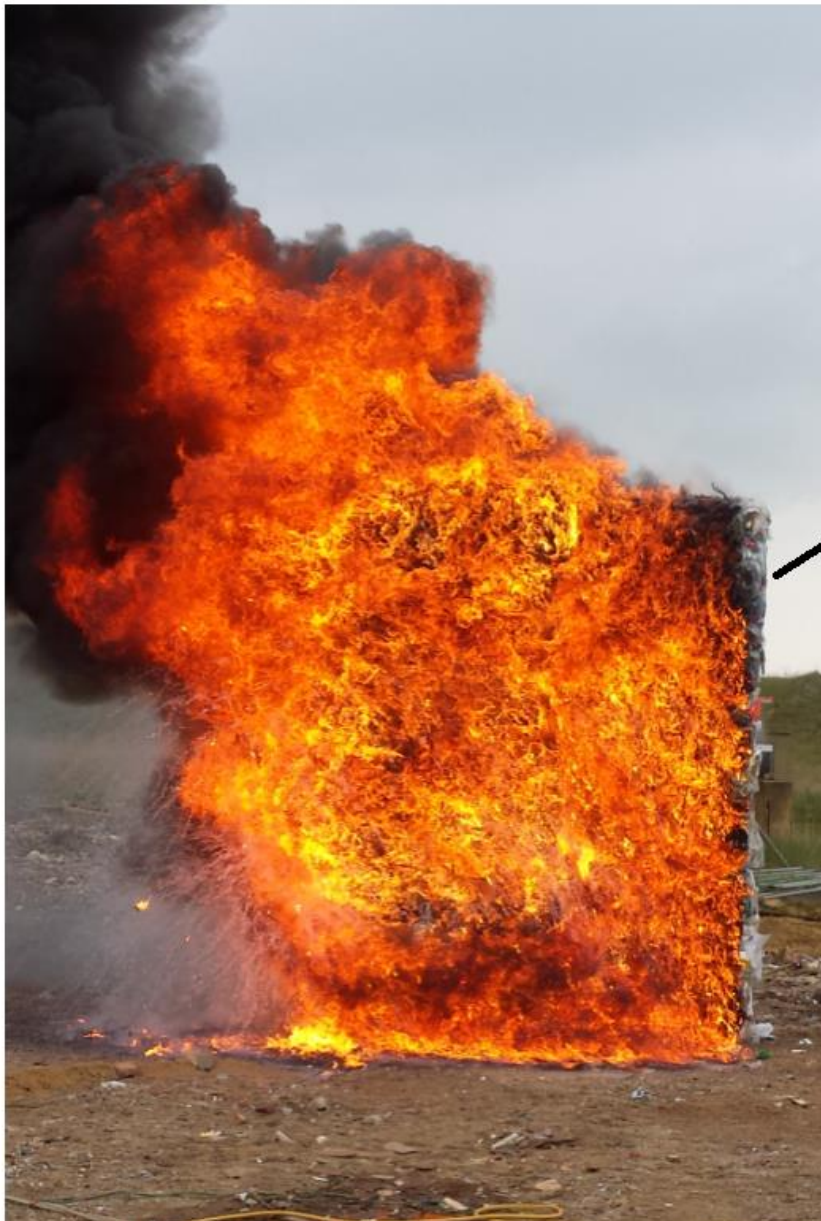
Figure 144 Test No 13 (table 2) HDPE clockwise fire spread
