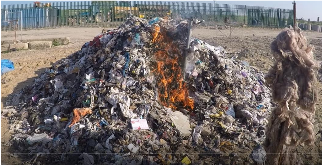
Figure 57: Test No 12 (table 2) fire fails to take hold at the core but spread to the surface
