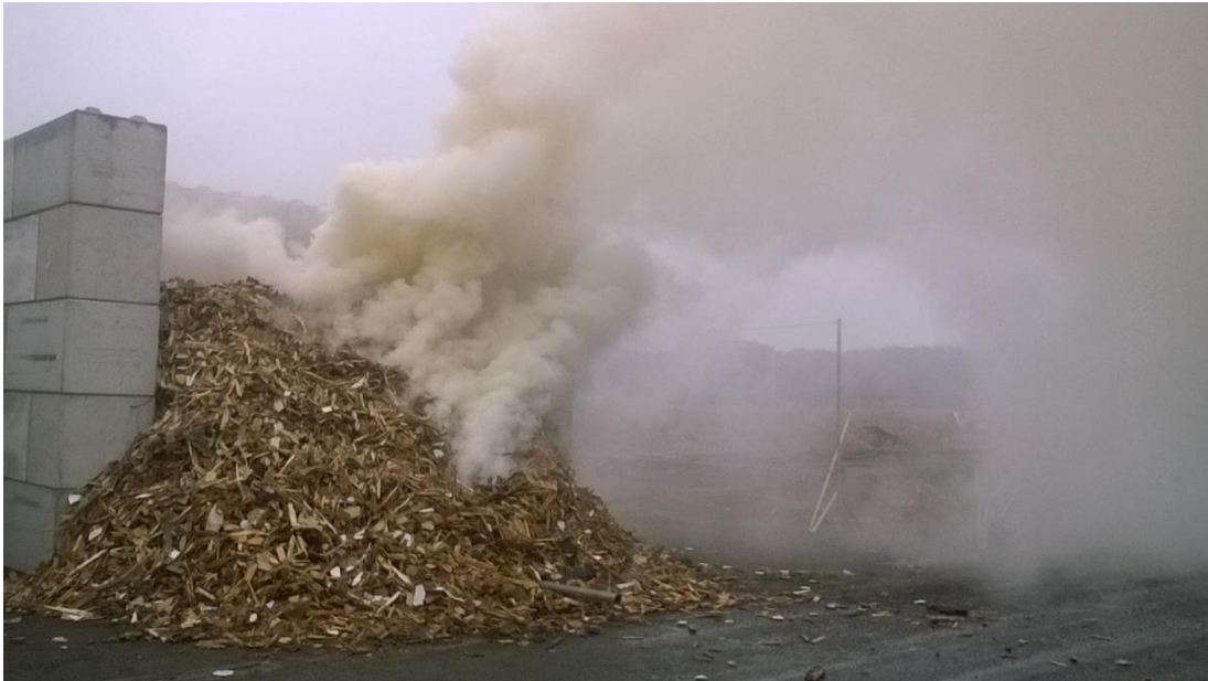
Figure 75: Test No 19 (table 2) smoke emission just before the flame breached the surface
