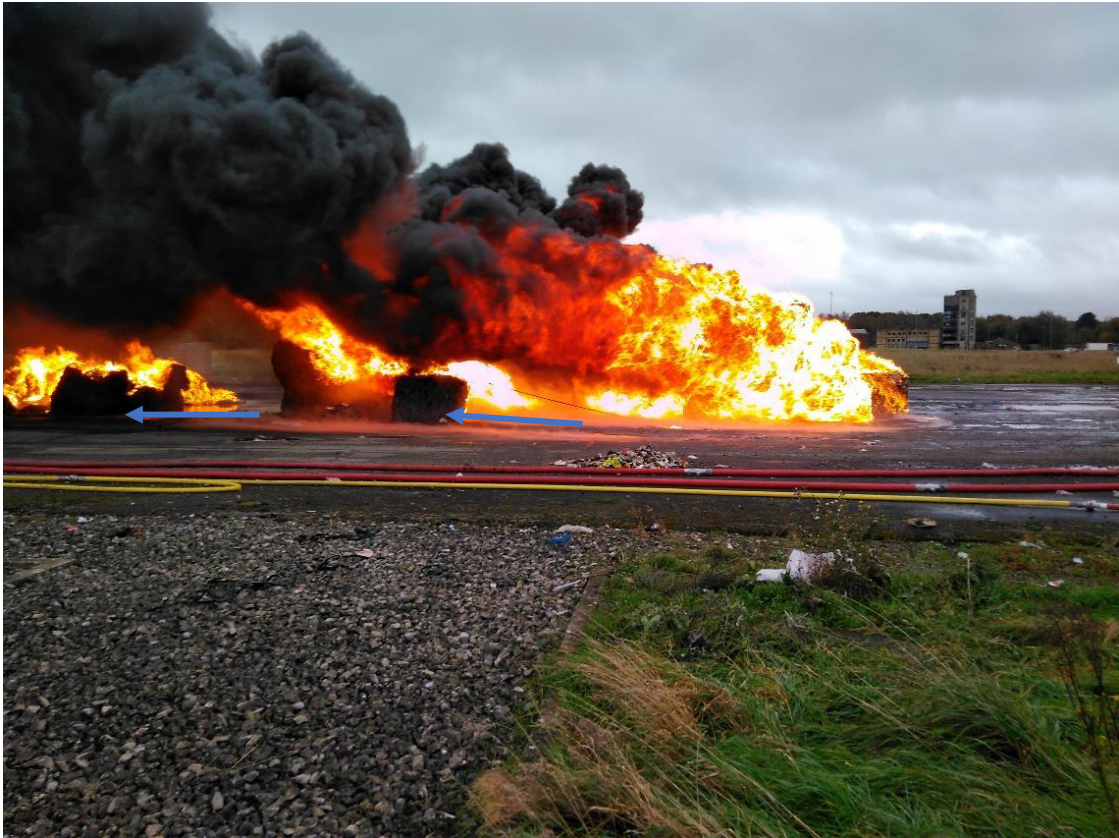
Figure 193: Test No 22 with two target fire to time fire spread between targets 6 m apart
