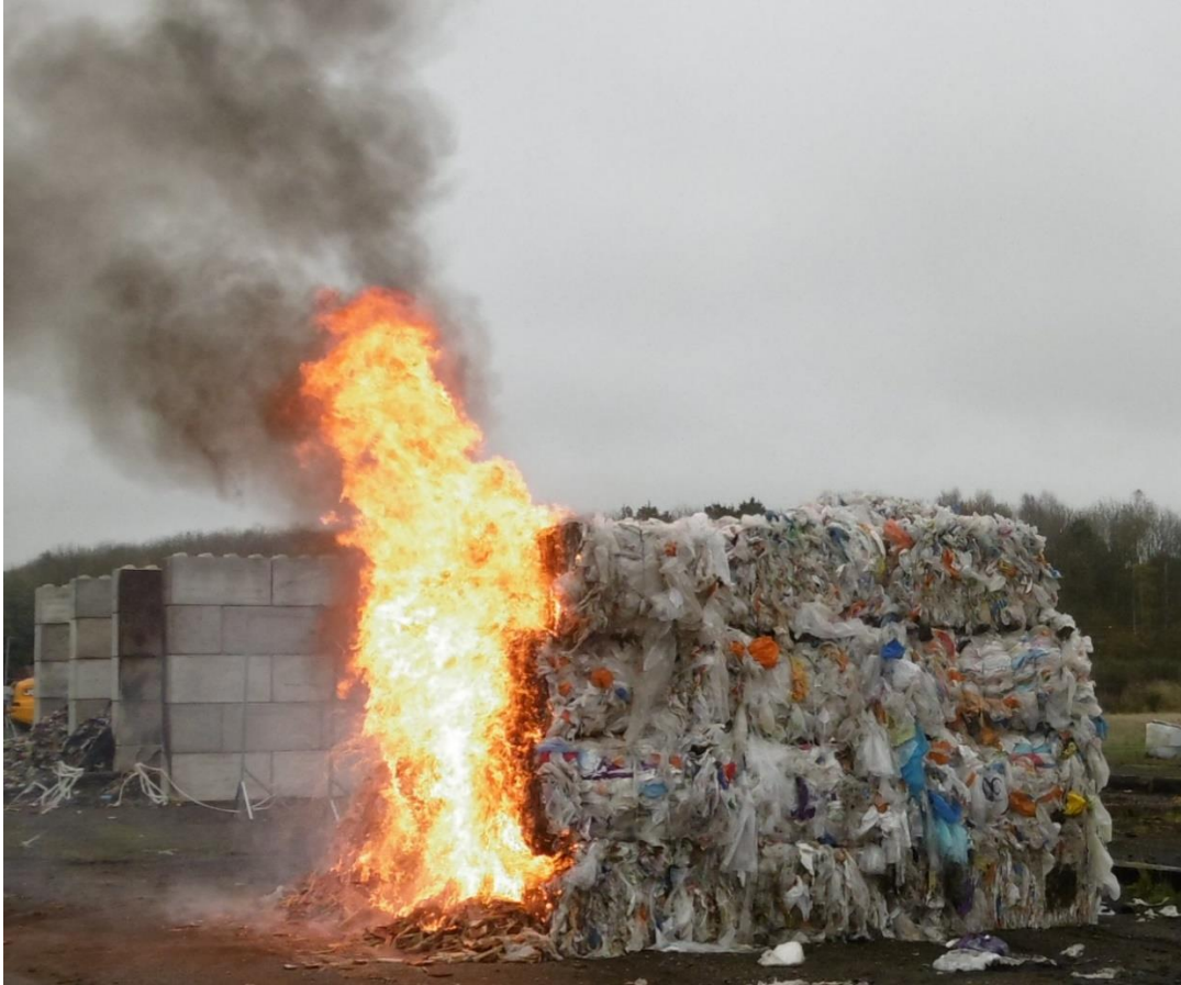
Figure 152: Test No 20 (table 2) Low Grade plastic fire vortex has formed
