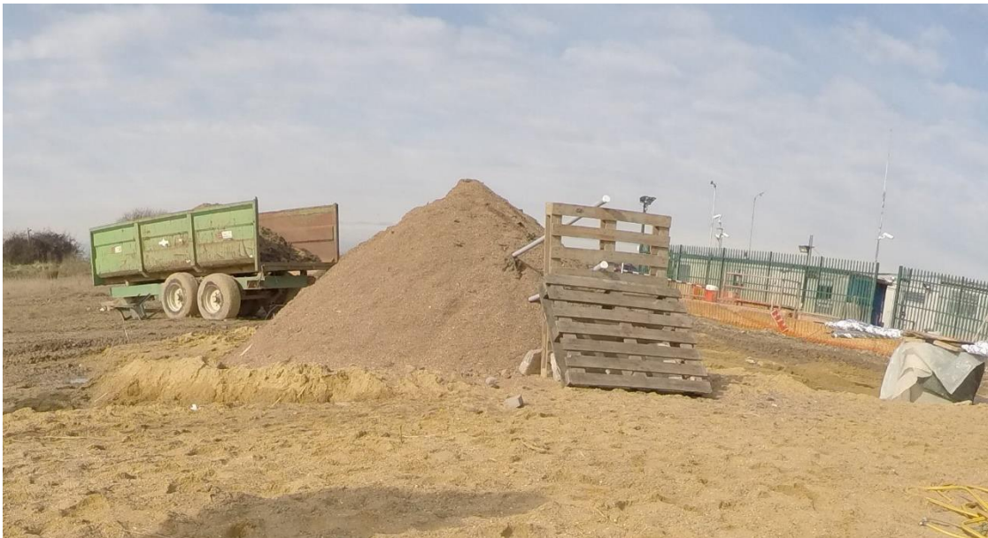
Figure 43: Test No 18 (table 2) wood fines self-heating test
