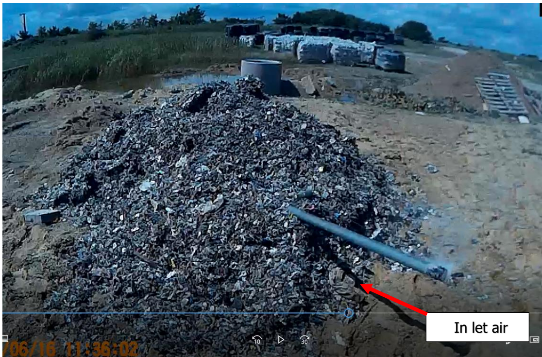
Figure 62: Test No 15 (table 2) deep seated SRF fire test
