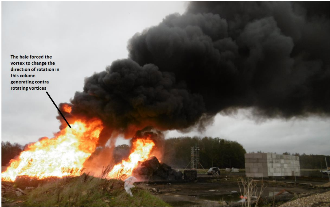
Figure 159: Test No 21 (table 2) Low grade plastic fire with anti-clockwise rotation vortex
