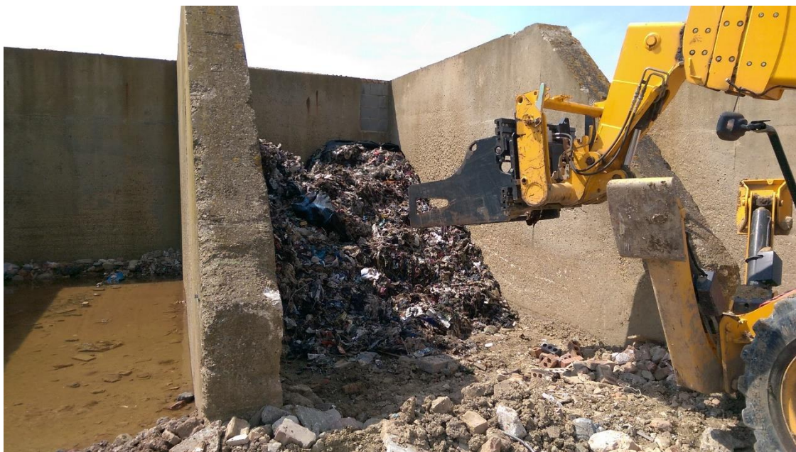
Figure 43: Test No 18 (table 2) wood fines self-heating test
