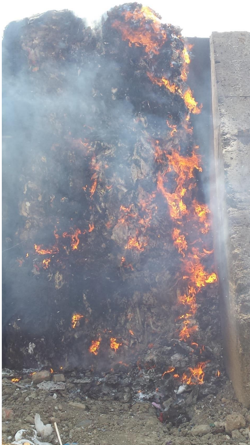
Figure 136: Test No 10 (table 2) surface fire now spreading to second stack
