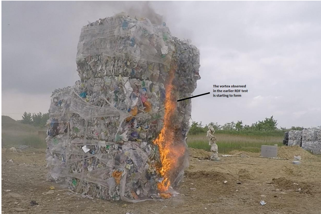
Figure 143: Test No 13 (table 2) HDPE test vortex forming
