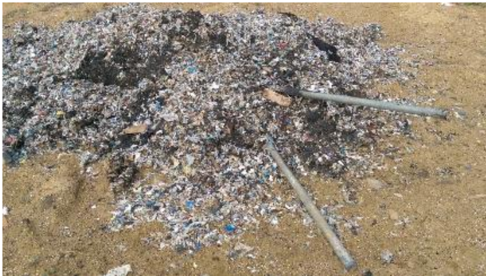
Figure 63: Test No 15 (table 2) SRF pile showing signs of self-heating
