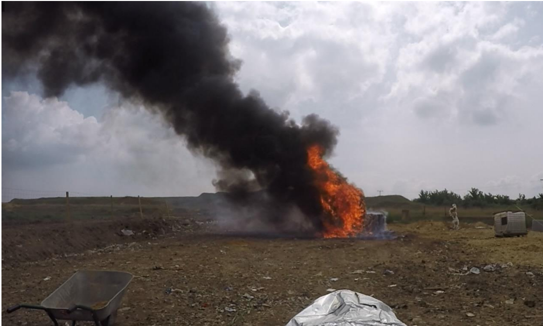
Figure 146: Test No 13 (table 2) HDPE fire vortex and smoke column
