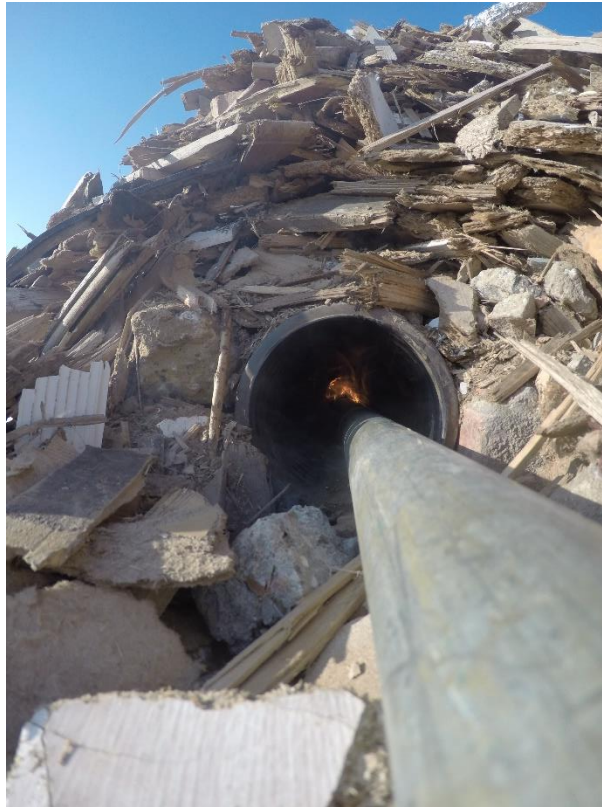
Figure 52: Test No 11 (table 2) deep seated wood fire test lighting at 07:50 am
