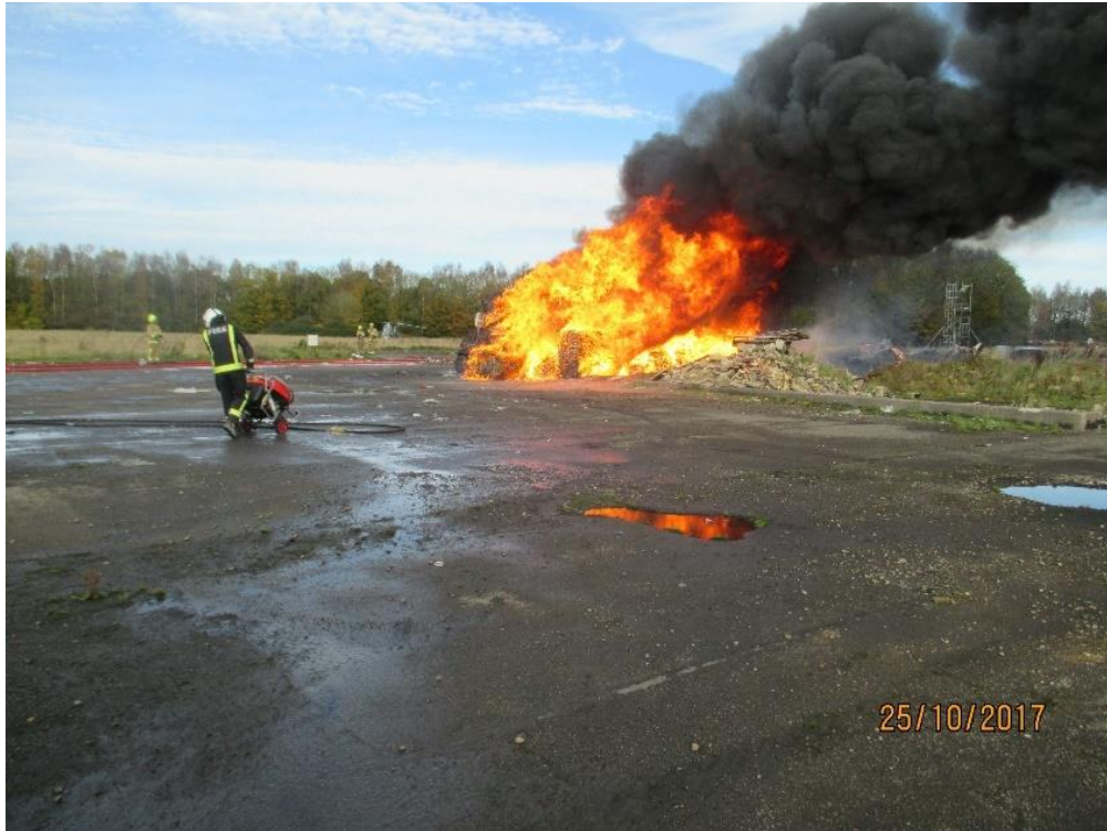
Figure 188: Low grade plastic. Surface temperatures are in excess of 1,100 °C
