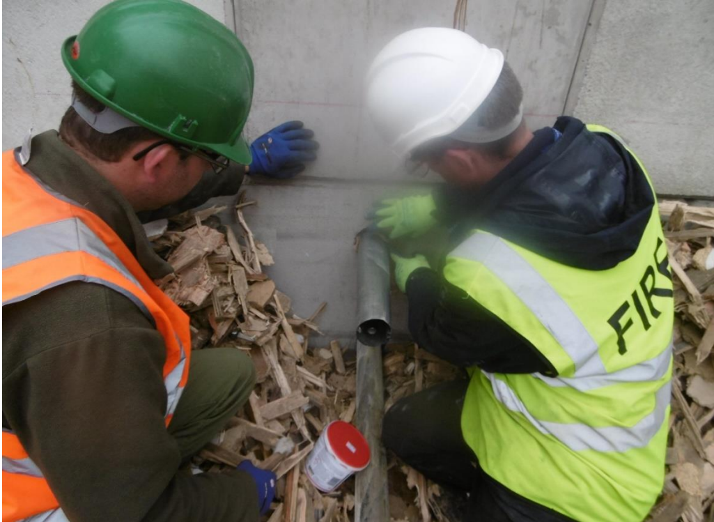
Figure 86: Test No 28(table 2) Setting up the igniter tube for deep seated RDF pile fire
