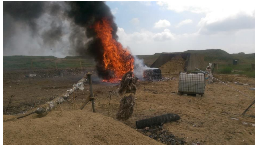
Figure 168: Plastic waste stacked bales resulting in flame temperature of 1200°C
