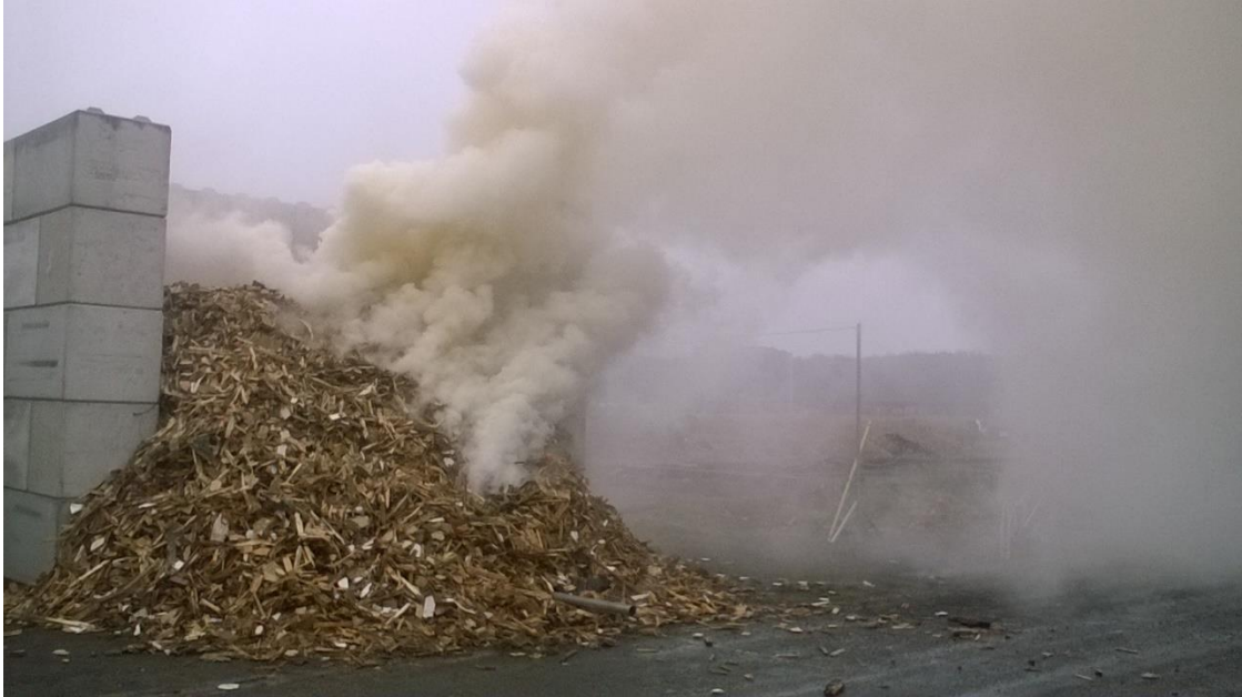
Figure 181: approximately 1 hour after ignition by 3 hours before breaching the surface
