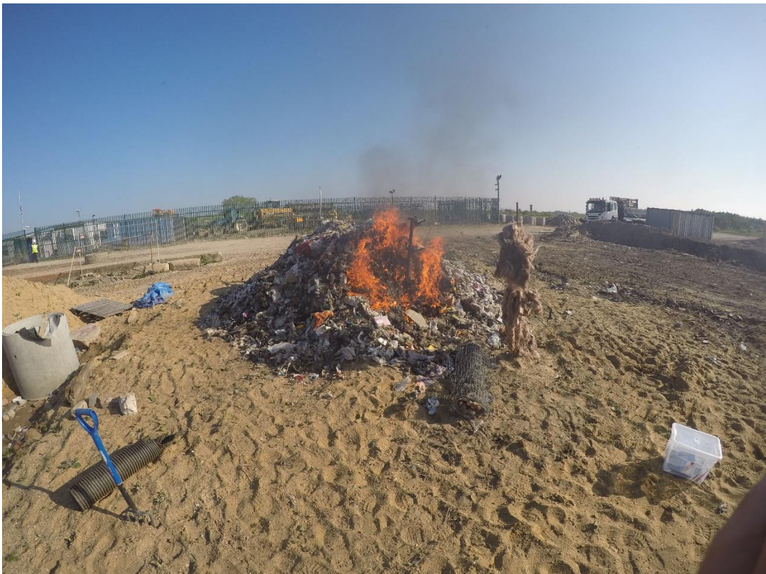
Figure 58: Test No 12 (table2) flame front can be seen moving away from the point of origin
