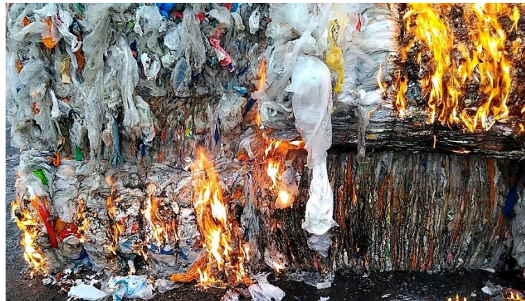
Figure 194: the bale of plastic ignited by the application of naked flame. The image is taken approximately 1 minute after ignition
