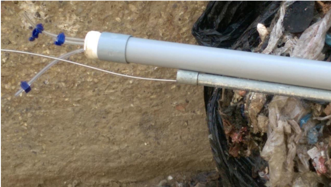
Figure 45: Gas sample tube and thermocouple for the RDF self-heating test
