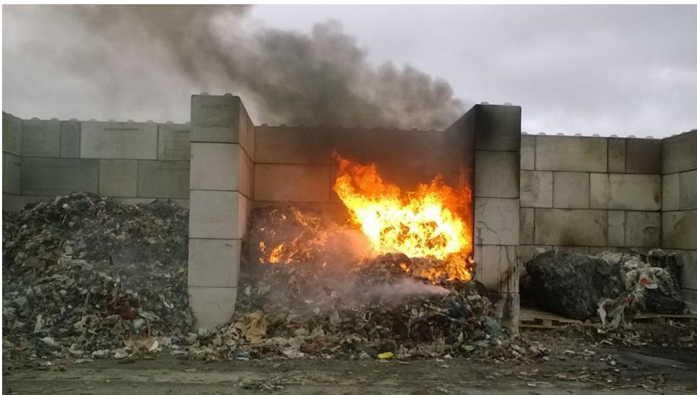
Figure 132: Test No 28a (table 2) Plastic Bay initiates a surface fire on RDF
