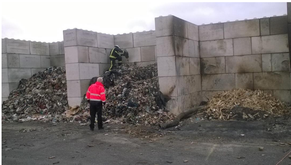
Figure 130: Test No 28a (table 2) diesel accelerant being applied
