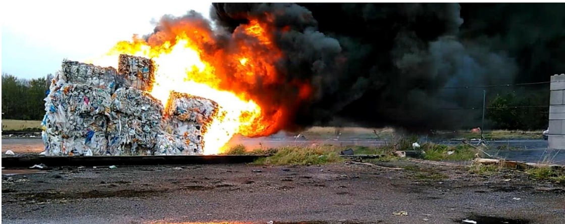
Figure 153: Test No 20n (table 2) Fire spread in a clockwise direction
