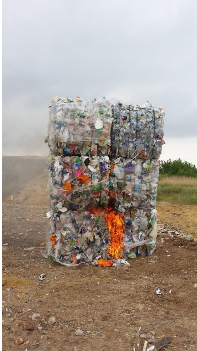
Figure 142: Test No 13 (table 2) HDPE fire takes hold
