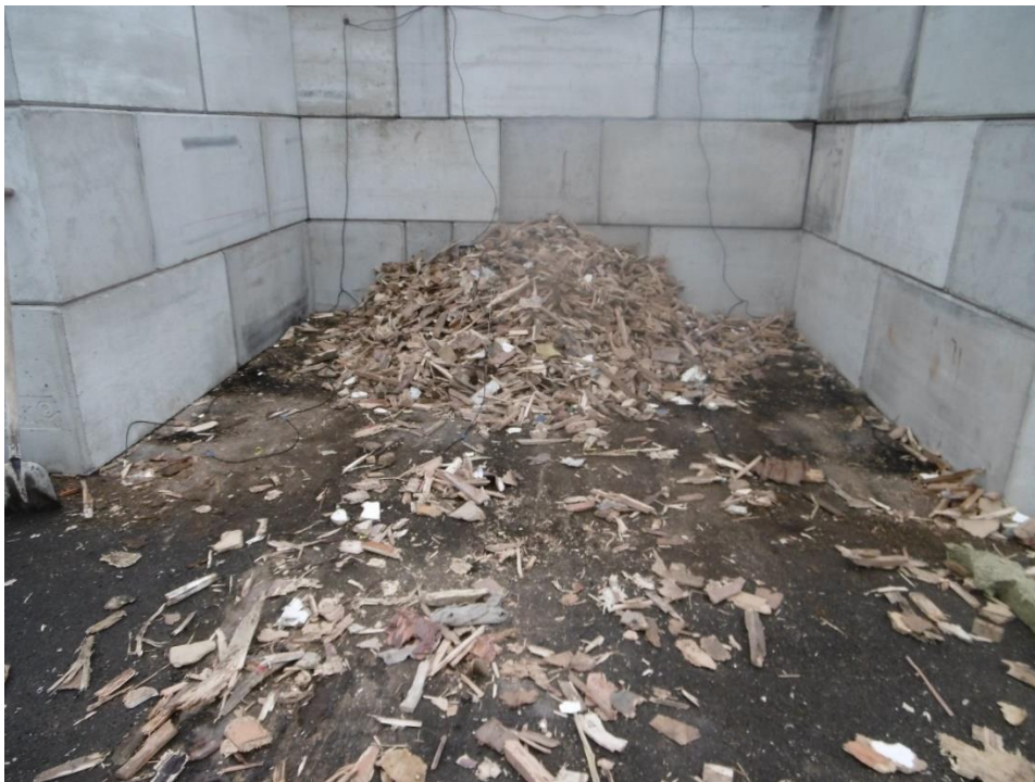
Figure 87: Test No 28 (table 2) Setting a timber pilot fire bed for the RDF fire
