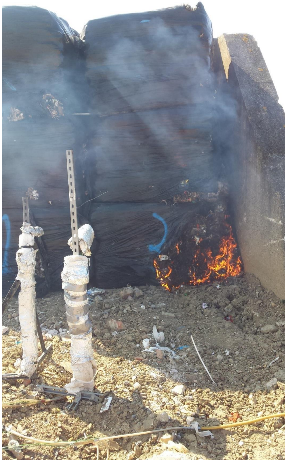
Figure 134 Test No 10 (table2) bale Fire developing with flame impingement on second vertical bale
