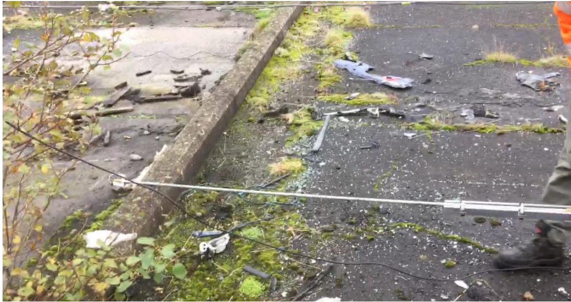
Figure 90: Oxi-propane lance supplied by Freeland Scientific Ltd (83)
