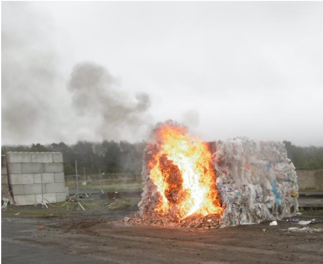
Figure 151: Test No 20 Low Grade plastic bale test
