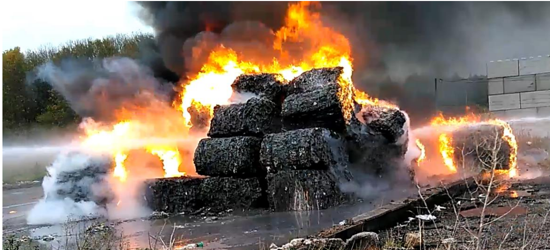
Figure 154: Test No 20 (table 2) Low grade plastic in the process of being extinguished with water see appendix F
