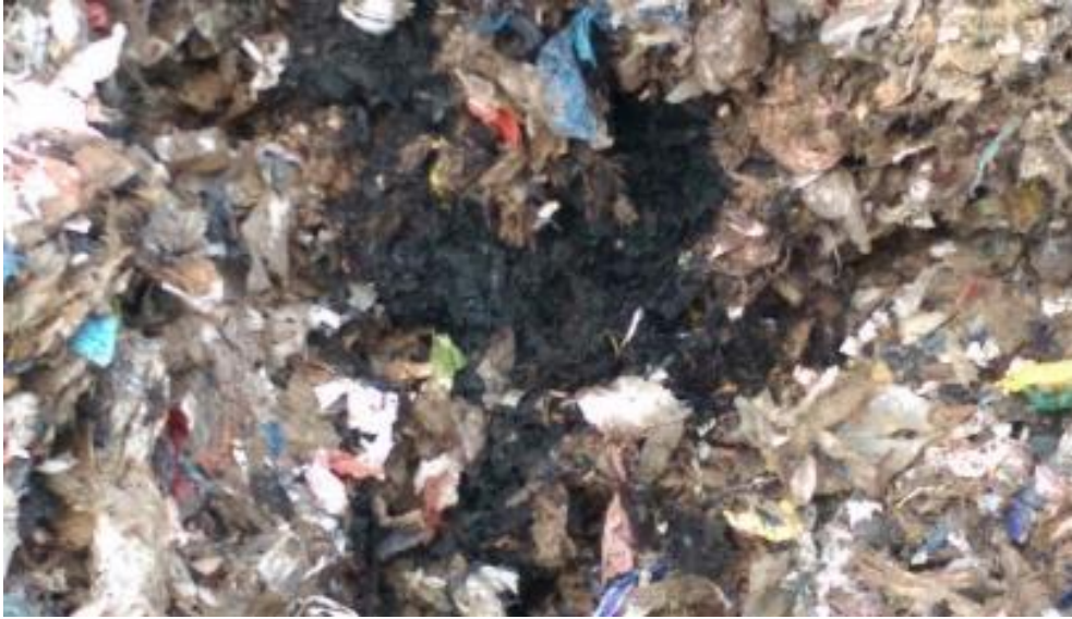
Figure 65: Test No 15 (table 2) self-heating zone exposed
