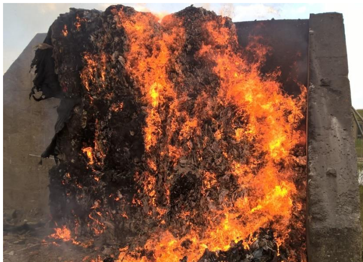
Figure 167: General wastes stacked bales resulting in flame temperature of 950°C
