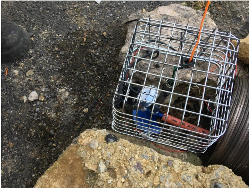
Figure 69: Test No 19 (table 2) Bunsen burner with a wireless detonator fuse
