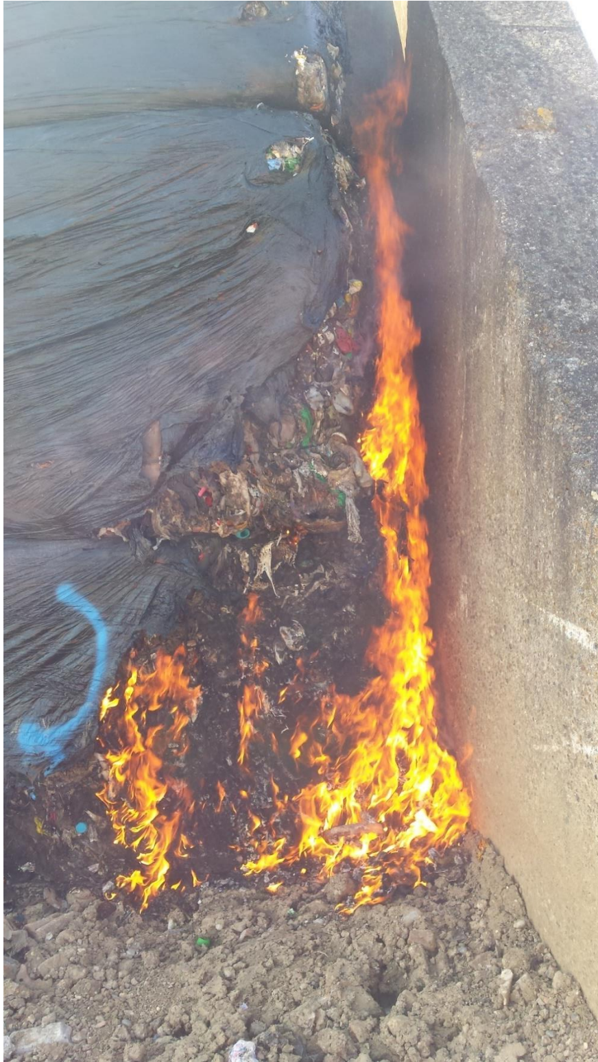
Figure 135: Test No 10 (table 2) RDF Bale Fire affecting third bale
