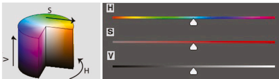
Fig. 4. Model of the HSV colour space. The left image is the courtesy of the author in (Rosebrock, 2017).
