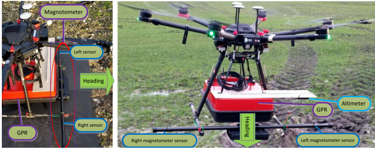
FIGURE 5: Onboard sensors: Magnetometer and GPR.
