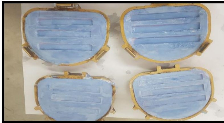
Fig. 2. Mold preparation for impact test specimens
