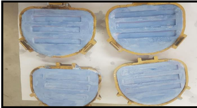
Fig. 2. Mold preparation for impact test specimens
