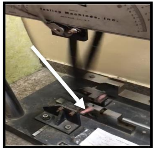
Fig. 4. After impact testing, a position the sample in the test device (Charpy type)
