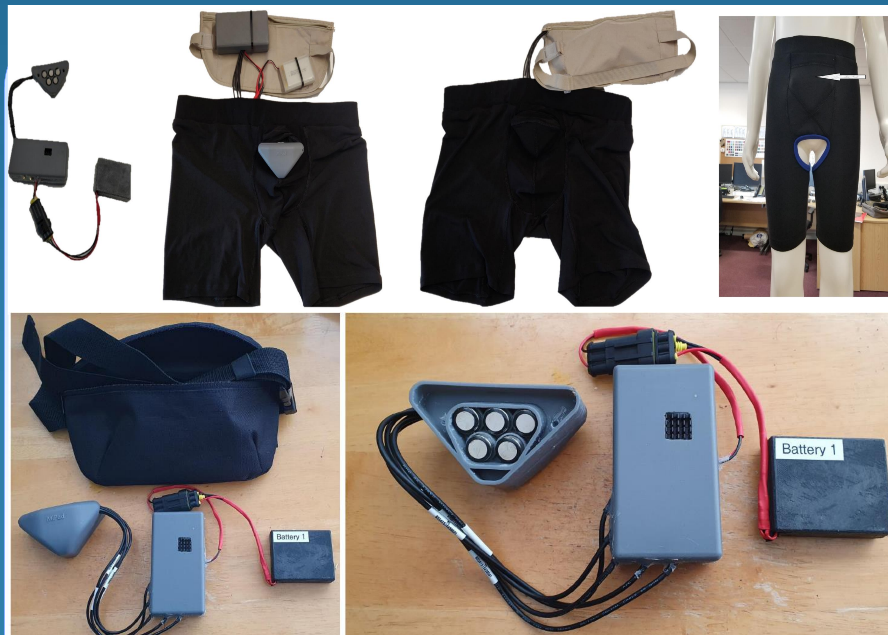
Figure 2. The advanced MyPAD device: i) US transmitter, ii) US receivers, iii) US electronics, iv) PCB, and v) AI unit. Top first version; Bottom last version.
