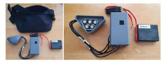
Fig. 3: The advanced MyPAD device: i) US transmitter, ii) US receivers, iii) US electronics, iv) PCB, and v) AI unit.
