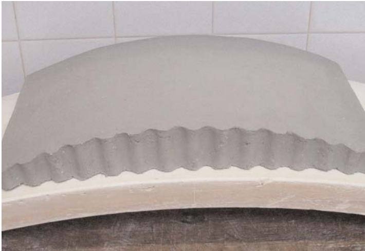
Pressed and shaped corrugated edged standing form.
