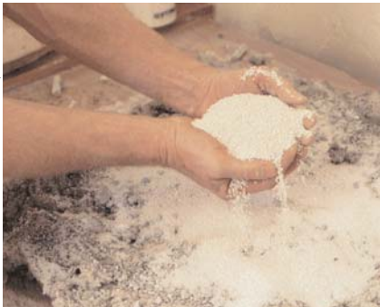
Adding molochite aggregate to a batch of porcelain.
