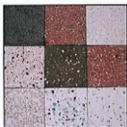
Examples of differing aggregate additions in clay bodies
