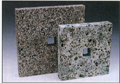
Pair of pierced forms made from kiln cast glass and ceramic aggregates (Binns 2007)
