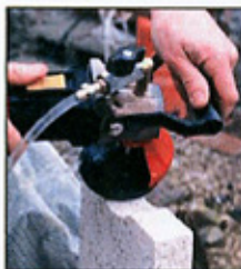
Flex Angle Grinder used to grind and polish fired forms
