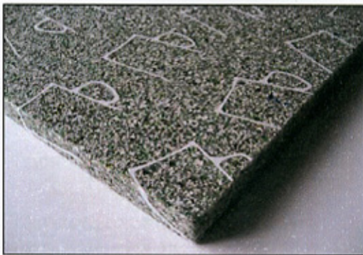
Slab of kiln cast glass and ceramic aggregates with cup 'fossils' (Binns & Bremner 2008)
