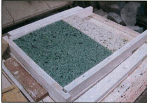
Kiln cast glass & ceramic aggregates using Refractory Concrete mould
