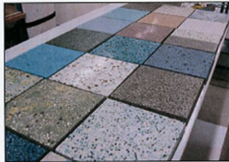
Test samples made from 97-100% fused glass, ceramic and mineral waste (Binns & Bremner 2010)
