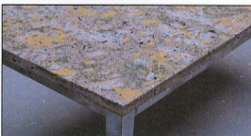
Detail of table top made from 97-100% fused glass, ceramic and mineral waste (Binns & Bremner 2010)
