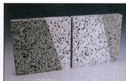
Two Piece Standing Form – Porcelain & kiln cast glass & ceramic waste (Binns 2008)
