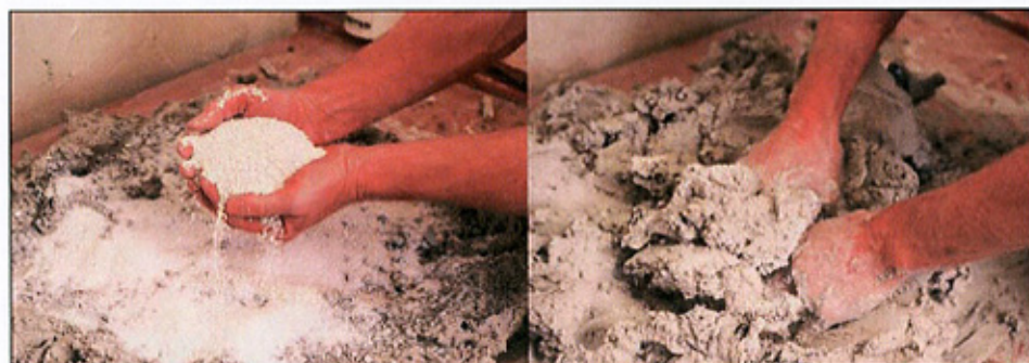
Hand wedging aggregates into plastic clay body
