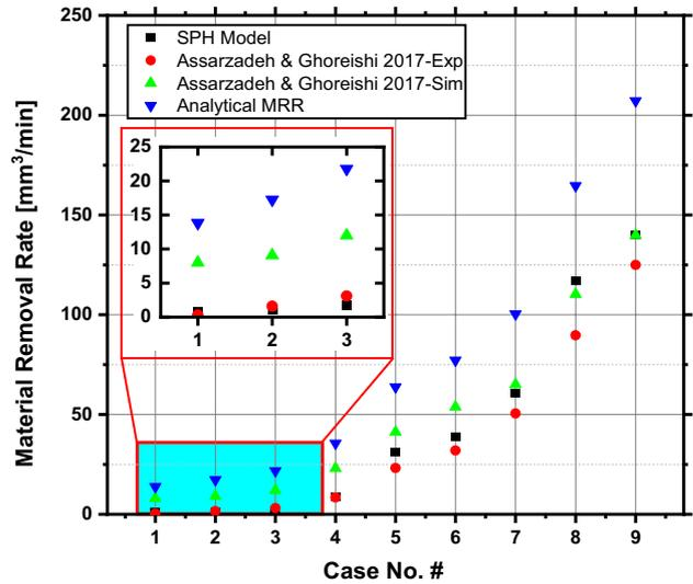
Fig. 19 MRR (mm<sup>3</sup>/min) for EDM of AISI 304 Steel using a constant discharge voltage of 25 V
