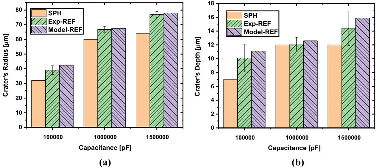
Fig. 11 Effect of process parameters on crater a radius and b depth compared to experimental and FEA results ( $V=220$  V,  $t_{ON}=5$   $\mu$ s) [8]
