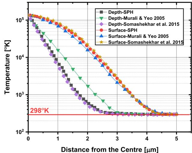
**Fig. 10** Temperature gradient along the surface and depth from the spark centre against [24] and [23]
