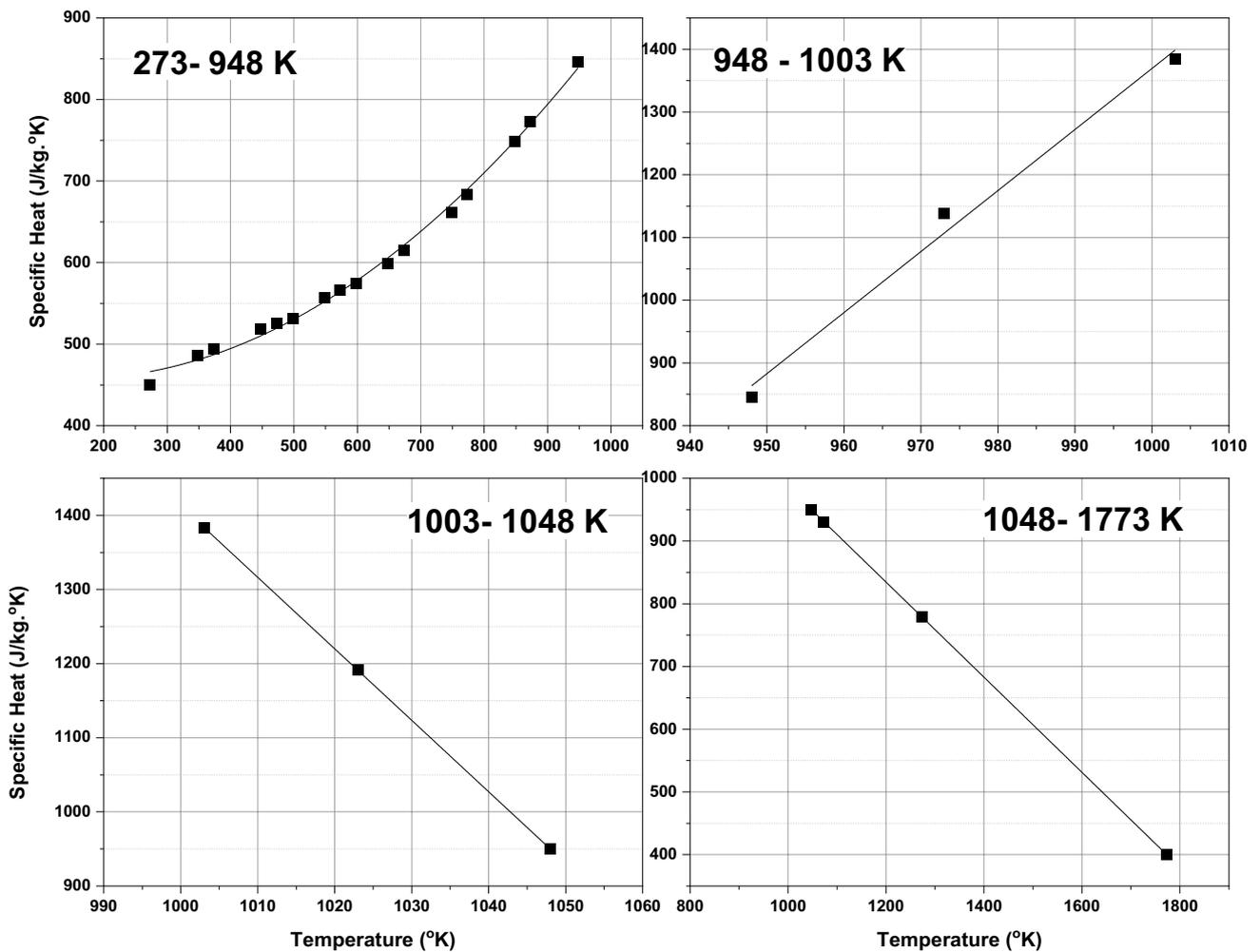
Fig. 3 Temperature-dependent specific Heat of AISI 304 alloy for a different range of temperature [39]
