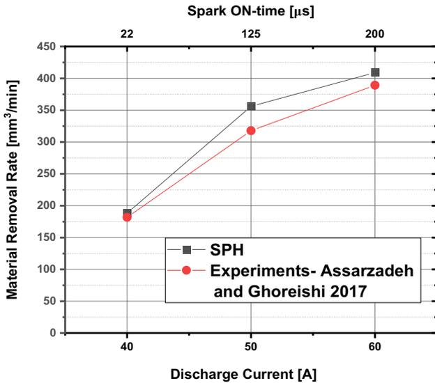
Fig. 18 Material removal rate comparison between SPH predictions and experiments
