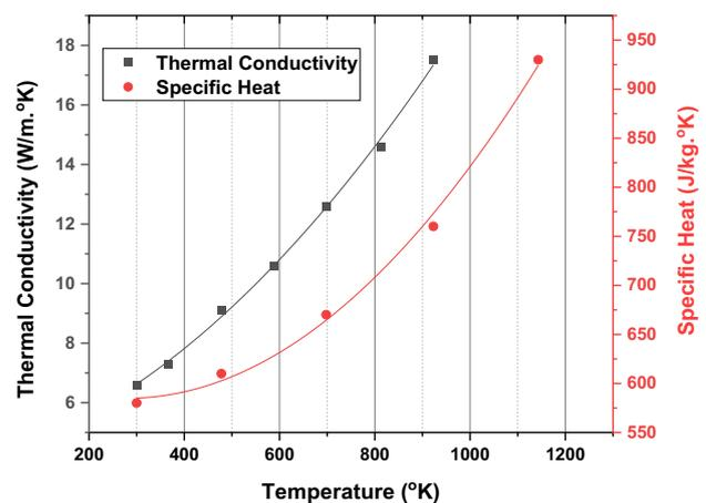
Fig. 1 Temperature-dependent thermal properties Ti-6Al-4V alloy [24]
