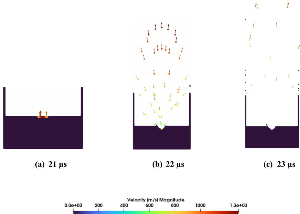
**Fig. 14** Machined material velocity field and the crater formed using 50 A and 125  $\mu$ s spark
