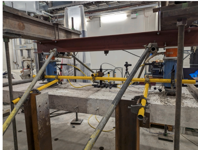
(b) View of the test frame showing the junction of the two types of concrete
