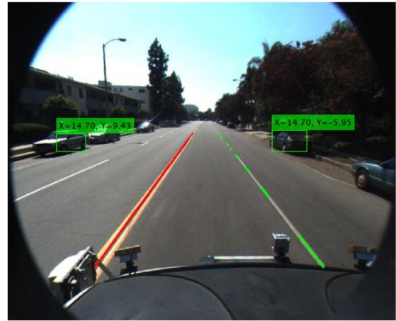
Fig. 11: SSA in Video 2 – instant relative positioning of other vehicles with respect to the ego vehicle.
